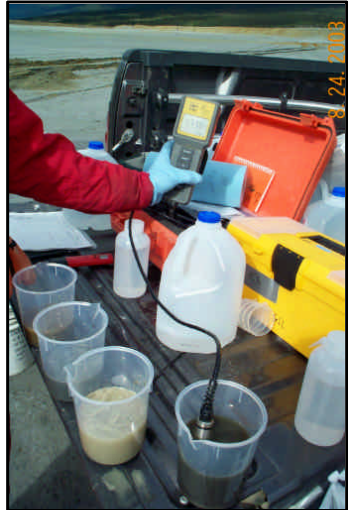
Field measurements of soil showing plastic beakers, soil slurry and field conductivity probe
