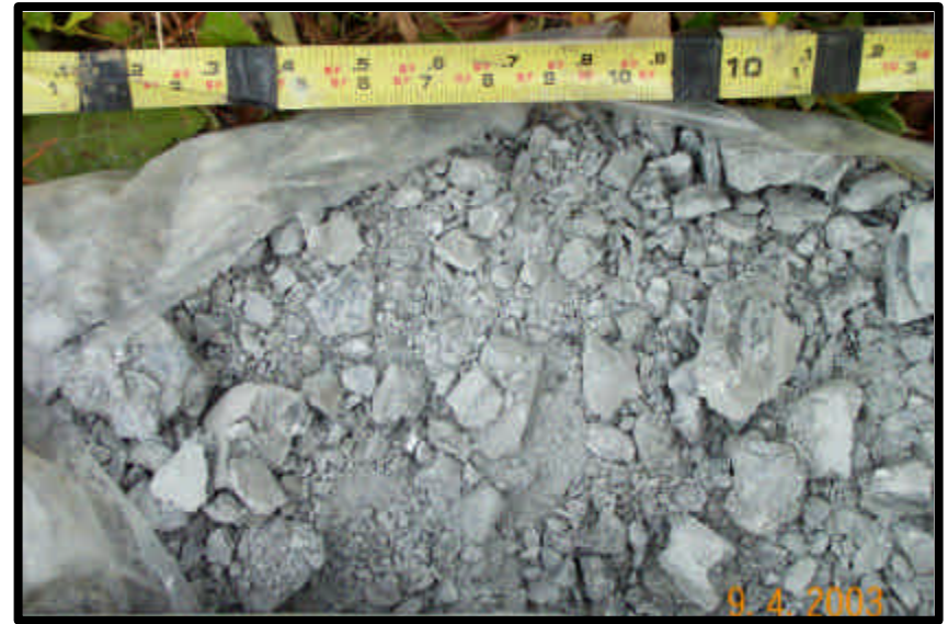
Identification of weathered bedrock
