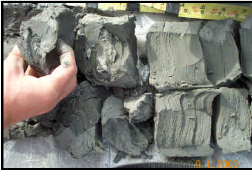
Core sample from P03-07 (155' - 165') showing lacustrine sediments (varved sequence)
