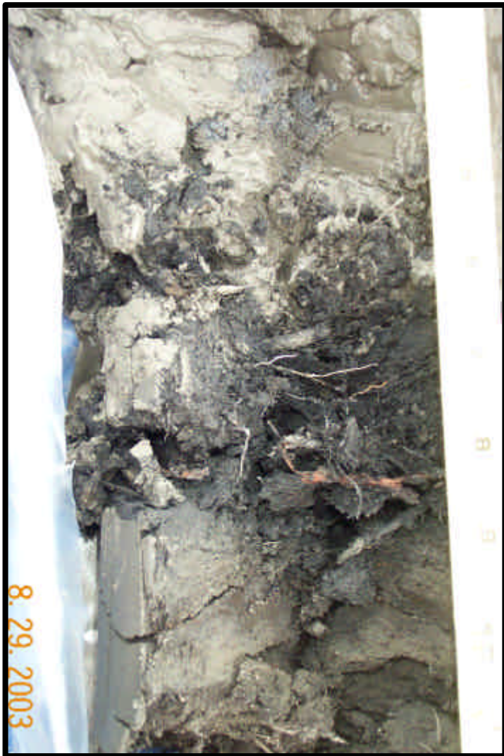
Detailed geology and identification of interface showing organics under the tailings
