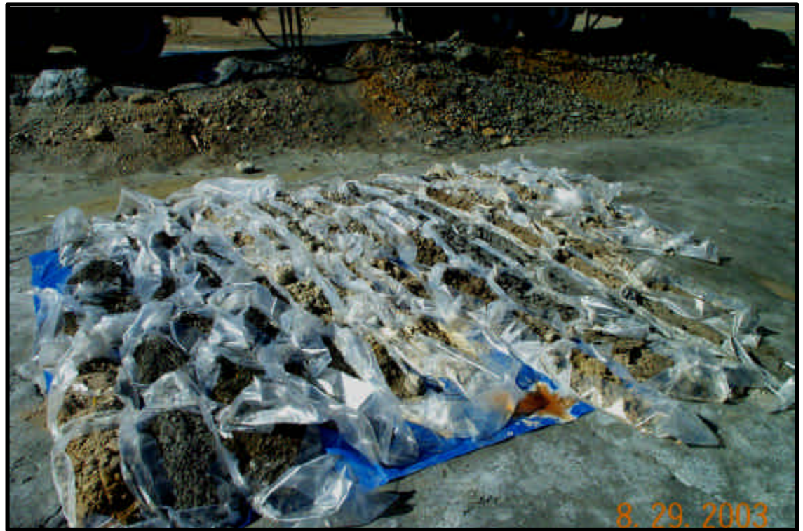
Cores at ground surface showing detailed geology and sharp transition in geological detail
