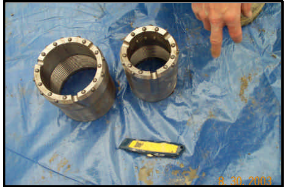
Outer casing and inner core barrel stainless steel shoe
