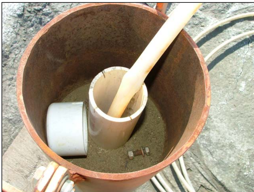
Well P01-08B (annular space filled with sand and sampling tubing stuck in well.)
