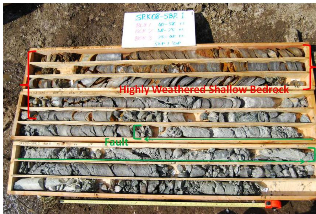
Photo 2: BR1 Core with Fault and Weathered Zone
