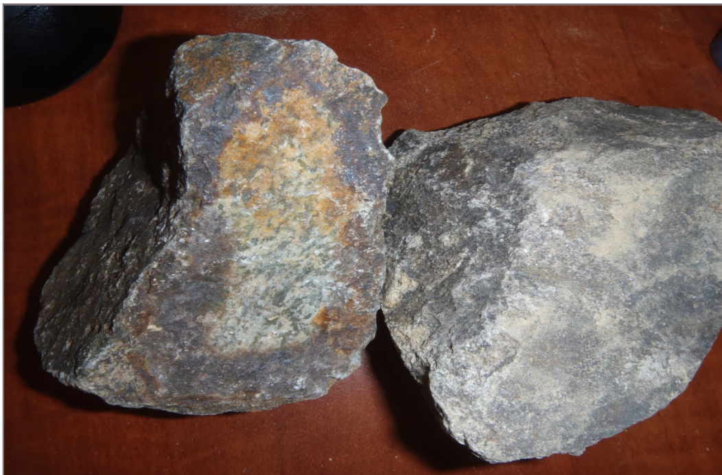
Photo 1: Sample 1 - note oxide staining. July 4, 2013
