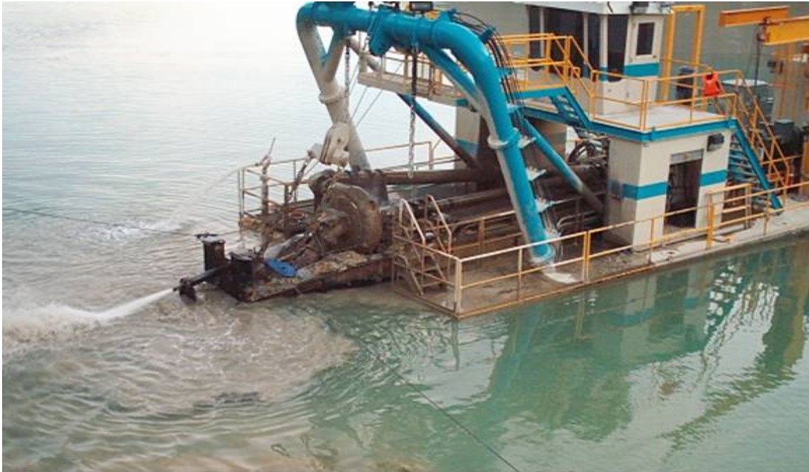
Figure 6.10: Suction dredge with cutter in action
