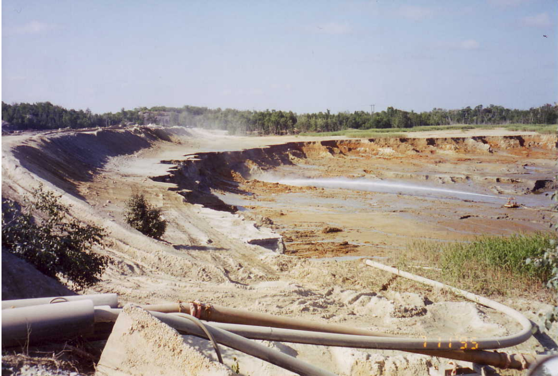
Figure 5.2: A hydraulic monitor working the bottom of a mining face
