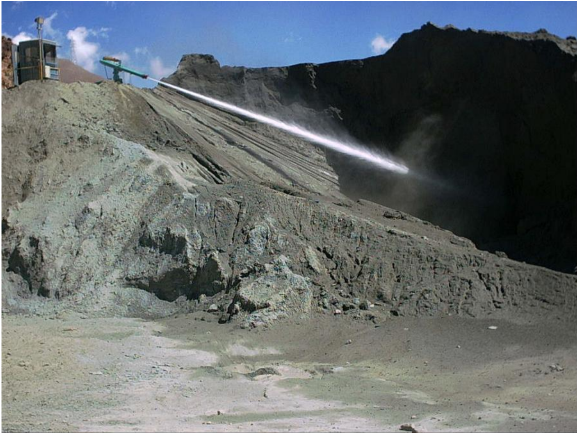
Figure 6.5: Hydraulic monitor in operation cutting a slope
