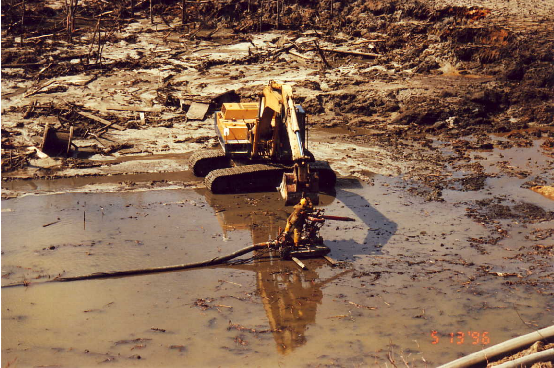
Figure 5.1: A hydraulic monitor being relocated closer to the mining face
