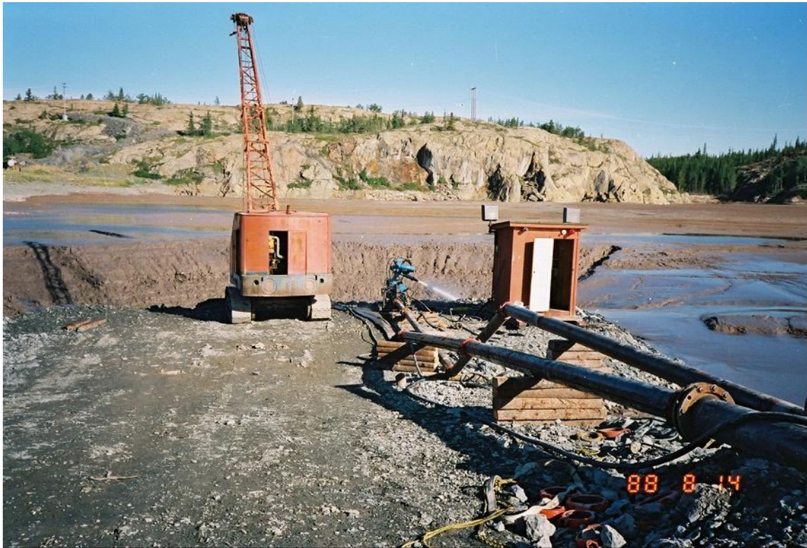
Figure 1.10: Initial mining setup in the Central Pond showing crane, monitor and operator's booth
