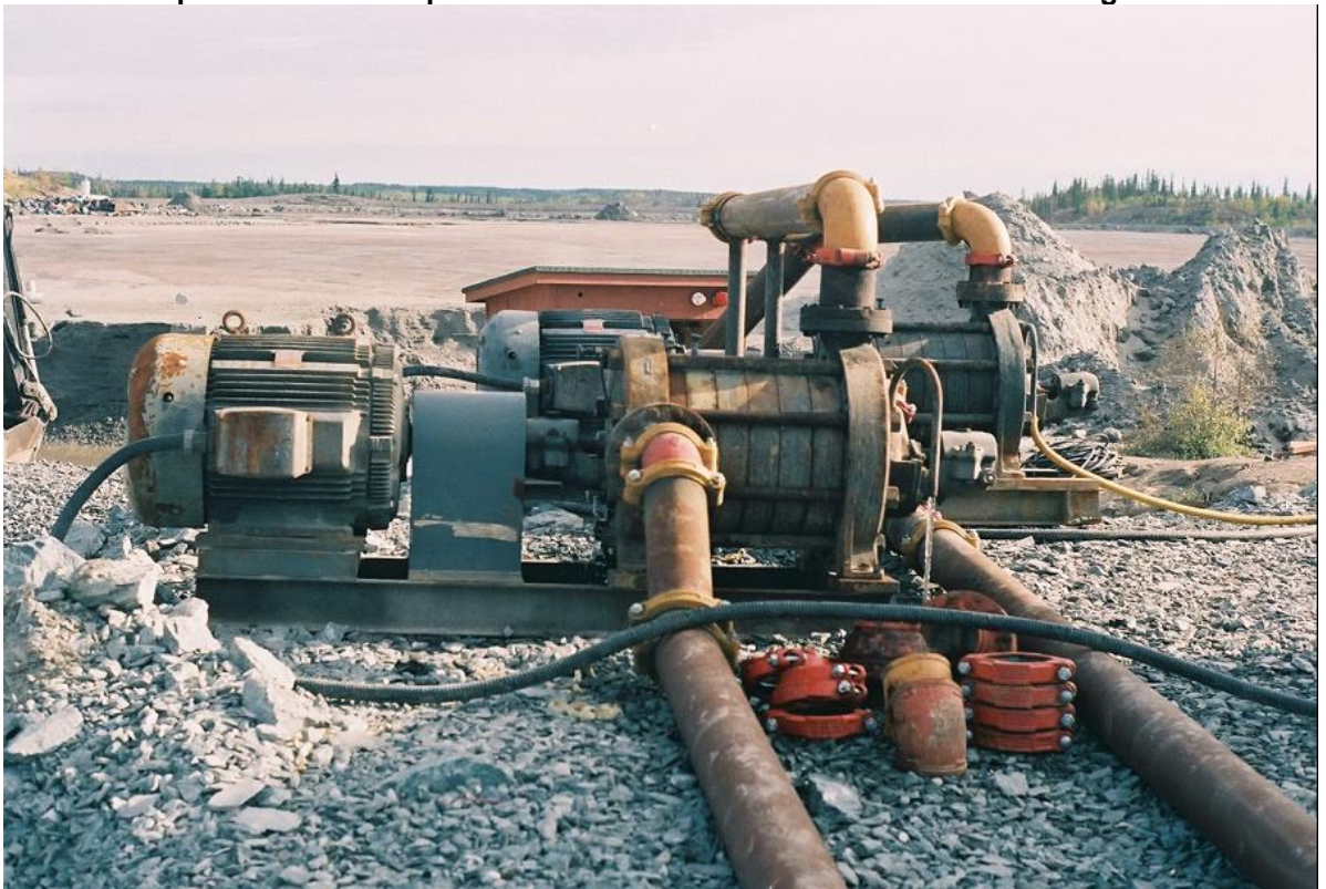
Figure 1.4: Mather+Platt multi-stage mine dewatering pumps connected in parallel used for high-pressure monitor feed water
