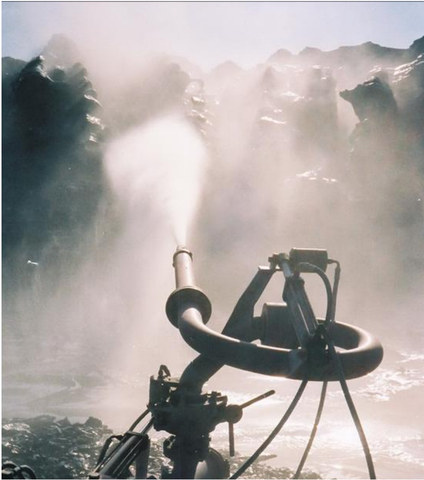
Figure 1.2: Hydraulic monitor washing frozen tailings
