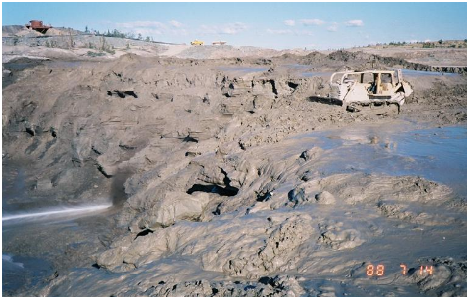
Figure 1.12: Dozer pushing thawed tailings to mining face
