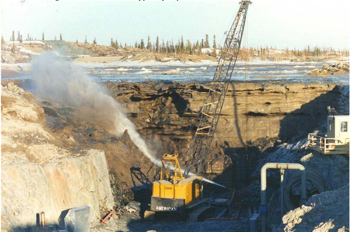
Figure 1.3: Start of the first ramp at Giant – May 1888. Note frozen tailings deflecting high pressure water. Operators booth and trommel screen are on the right.
