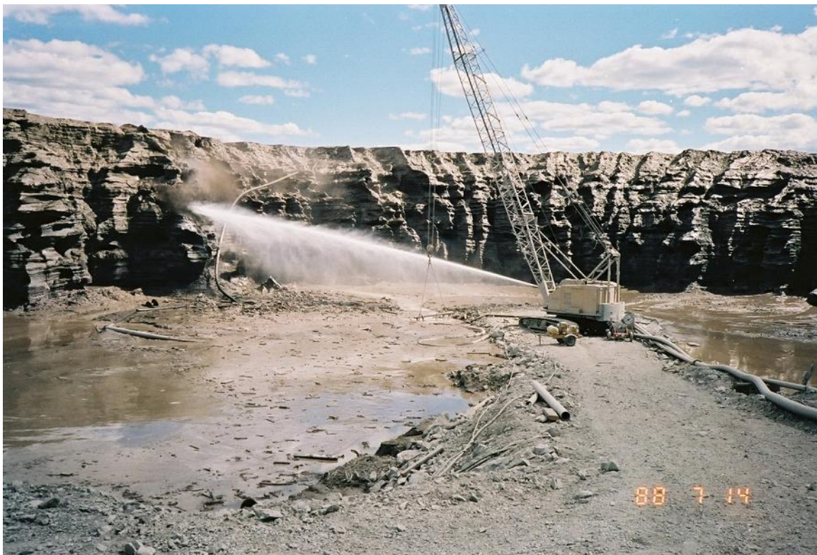
Figure 1.8: View of mining face showing monitor and crane.
