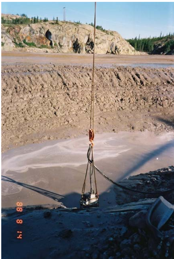
Figure 1.11; Toyo pump starting a sump in the Central Pond
