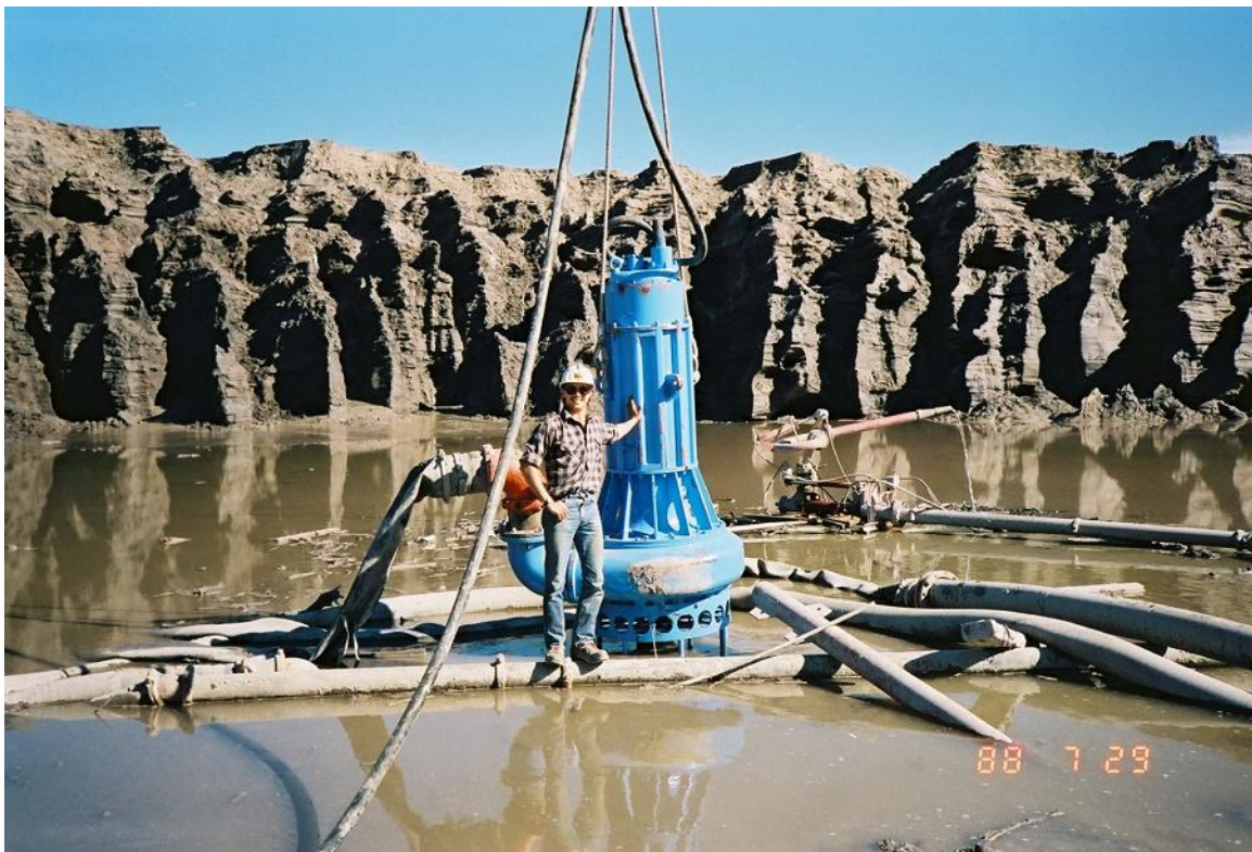
Figure 1.9: Toyo pump suspended from crane
