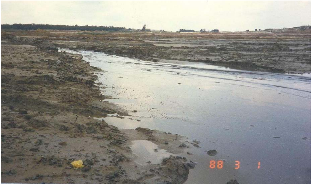
Figure 4.3 Slurry flowing from a mining face to a collection ditch at ERGO
