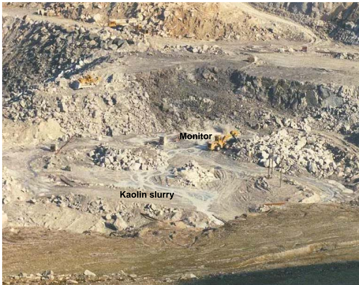
Figure 3.1: Dozer and loader moving waste rock while a monitor washes kaolin
