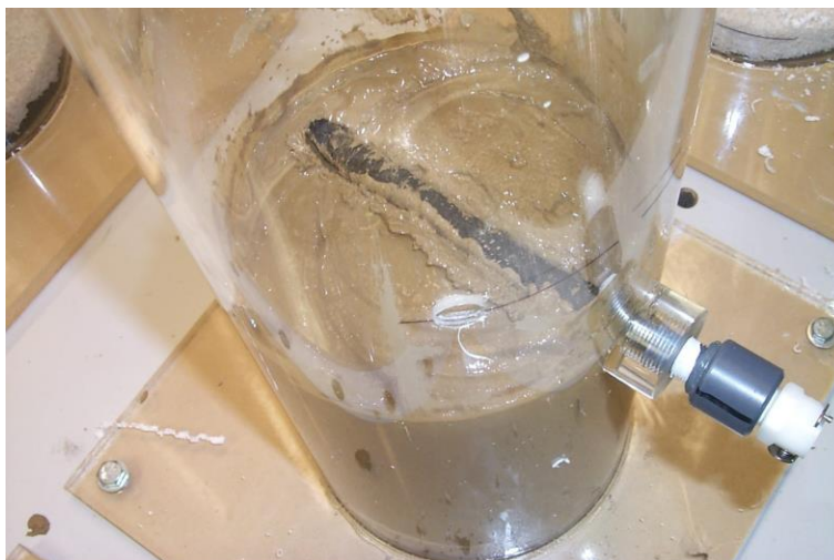
Figure 4: The sampling port for pore water samples.
