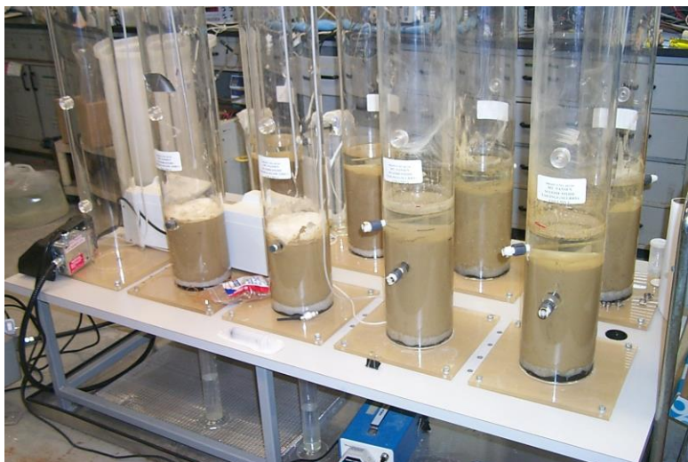
Figure 5: The eight columns set up to study the four disposal options
