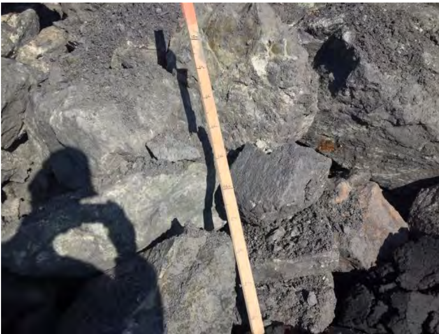
Large Diameter Rock (300-800mm in specs) – 1 of 5. Stick is 1 m long from tip to just below orange.
