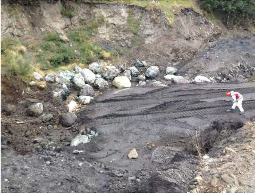
Looking north: Testing compacted waste rock. 20-24% m/c, 64-67% MPMDD. Material deemed not sufficient.
