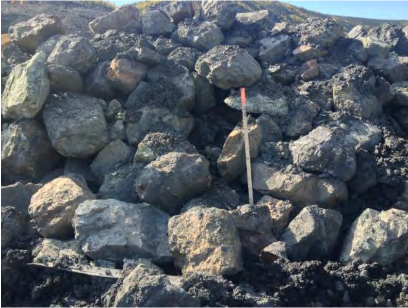
Large Diameter Rock (300-800mm in specs) – 4 of 5
