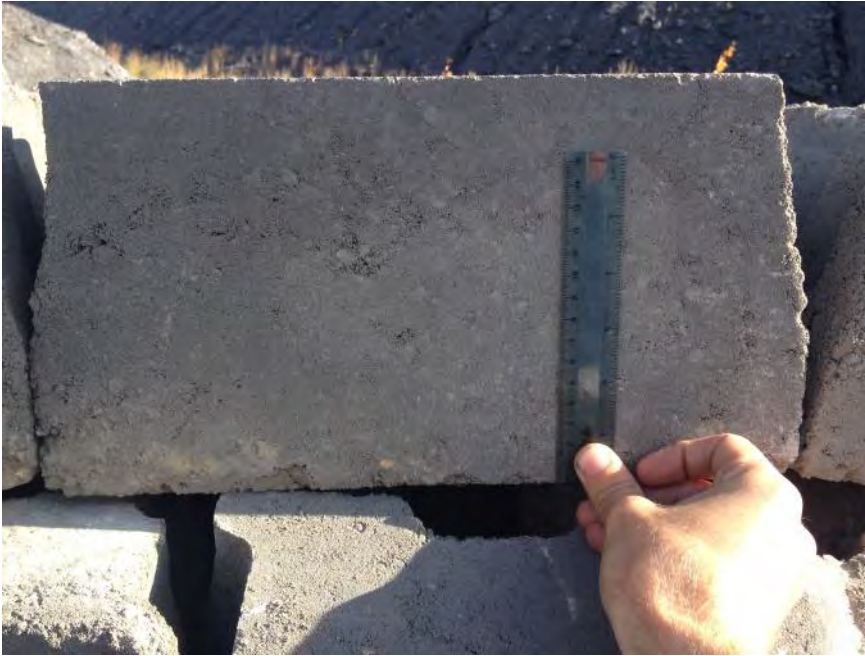
Armorflex mats: Pretty close to 190 cm block height.
