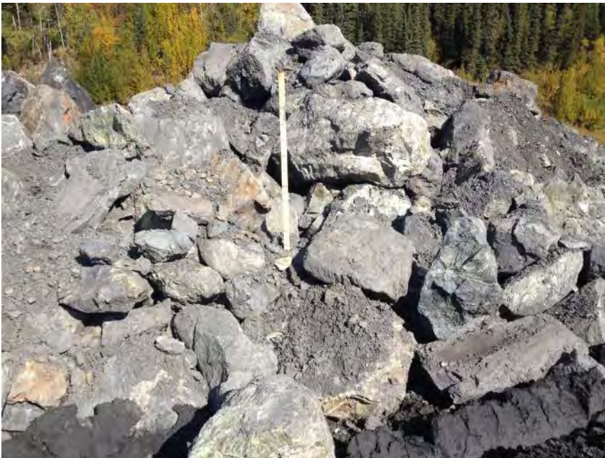
Large Diameter Rock (300-800mm in specs) – 5 of 5
