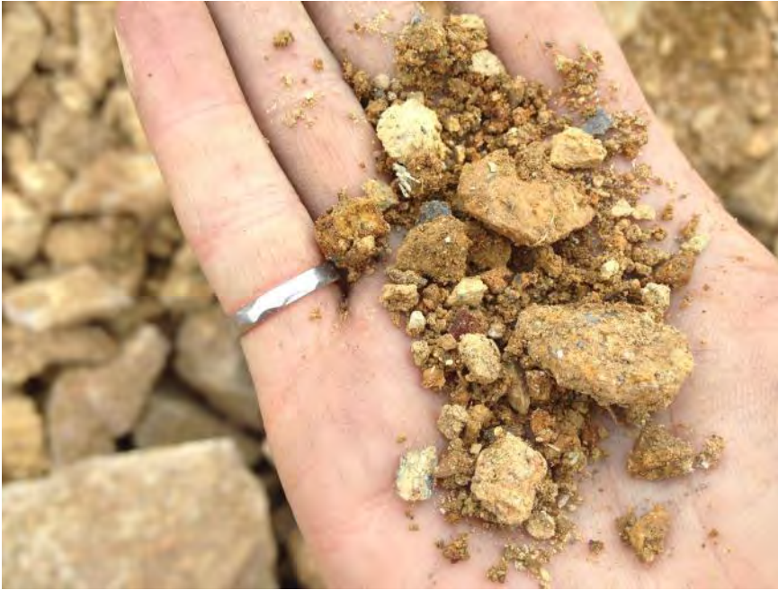
Proposed new channel fill. Granular, no cohesiveness.
