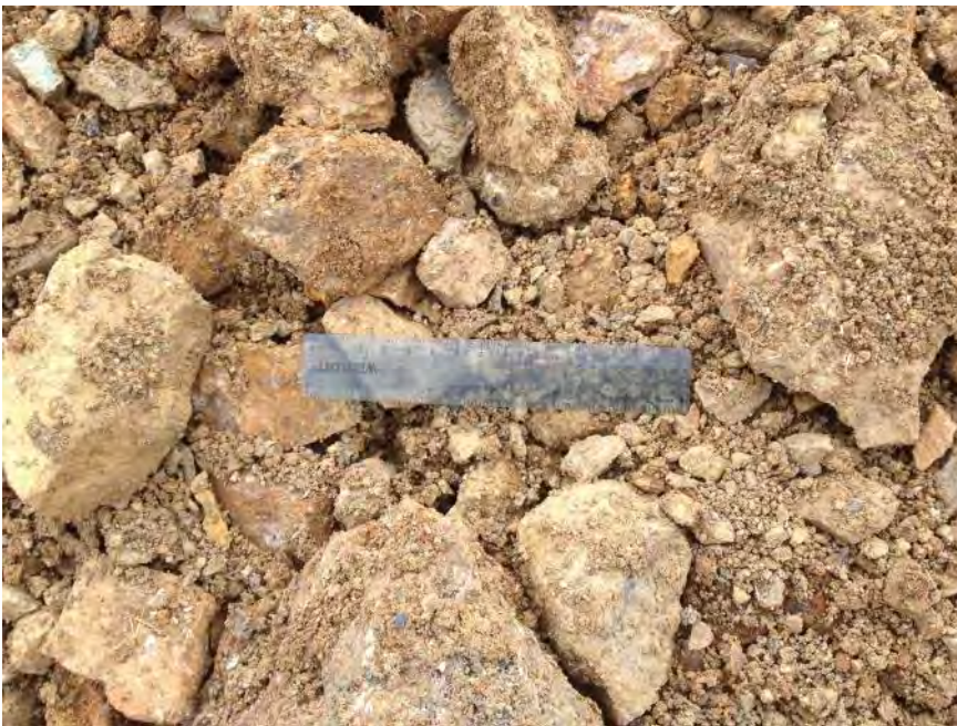
Proposed new channel fill. Same appearance as 100mm minus at Entrance Pit, but larger rocks, few fines.
