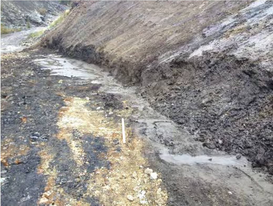
Looking east: ~1 L/s seepage of water from toe. Assumed to be rainwater running along top of permafrost. Delta of fine sediment deposited in background.
