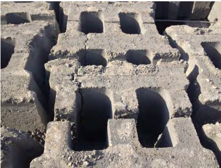
Armorflex mats: Crack through that will need repair. Only defect found in top mat on stack.
