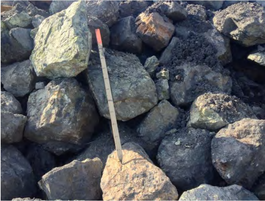
Large Diameter Rock (300-800mm in specs) – 2 of 5
