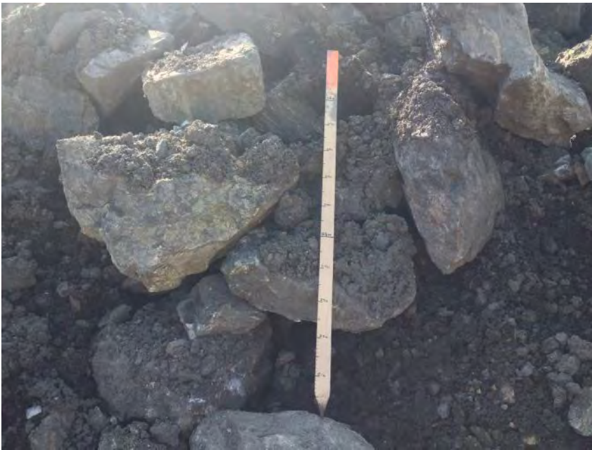
Large Diameter Rock (300-800mm in specs) – 3 of 5
