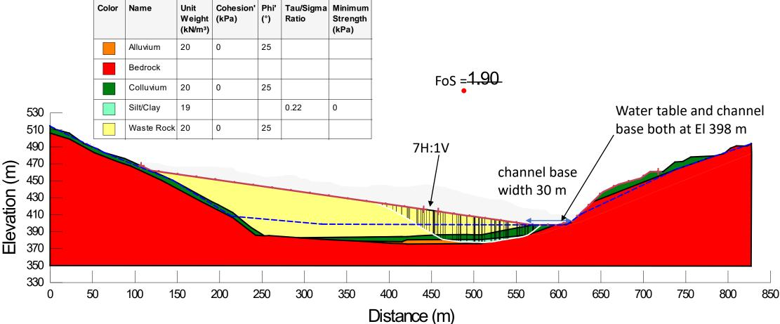
Option CC2 - Lake at El. 400 m Spillway Design Construction – Static liquefaction
