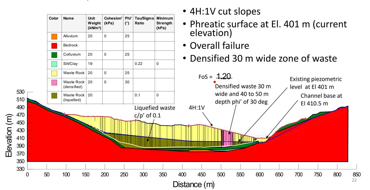
Scenario CC1 - Lake at El. 412 m Spillway Design Construction – Static liquefaction 6H:1V South Side Spillway Channel Slope
