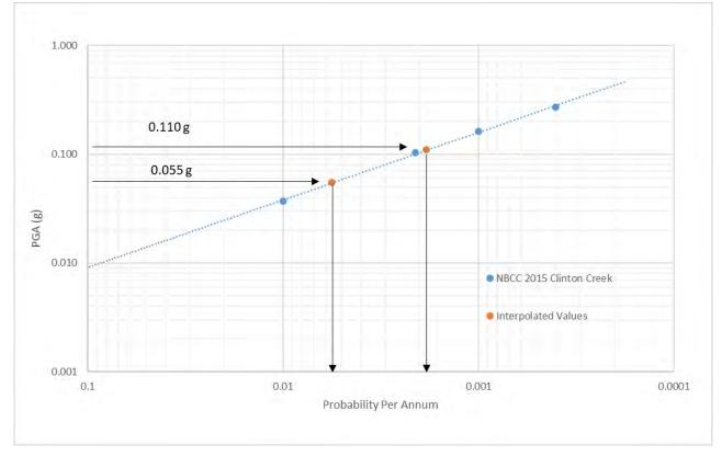
Figure 1: Annual Probability of Seismic Hazard at Clinton Creek
