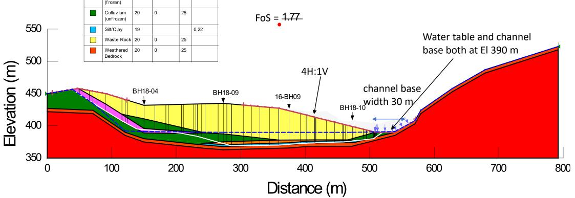
Option CC2 - Lake at El. 400 m Spillway Design Construction – Static liquefaction
