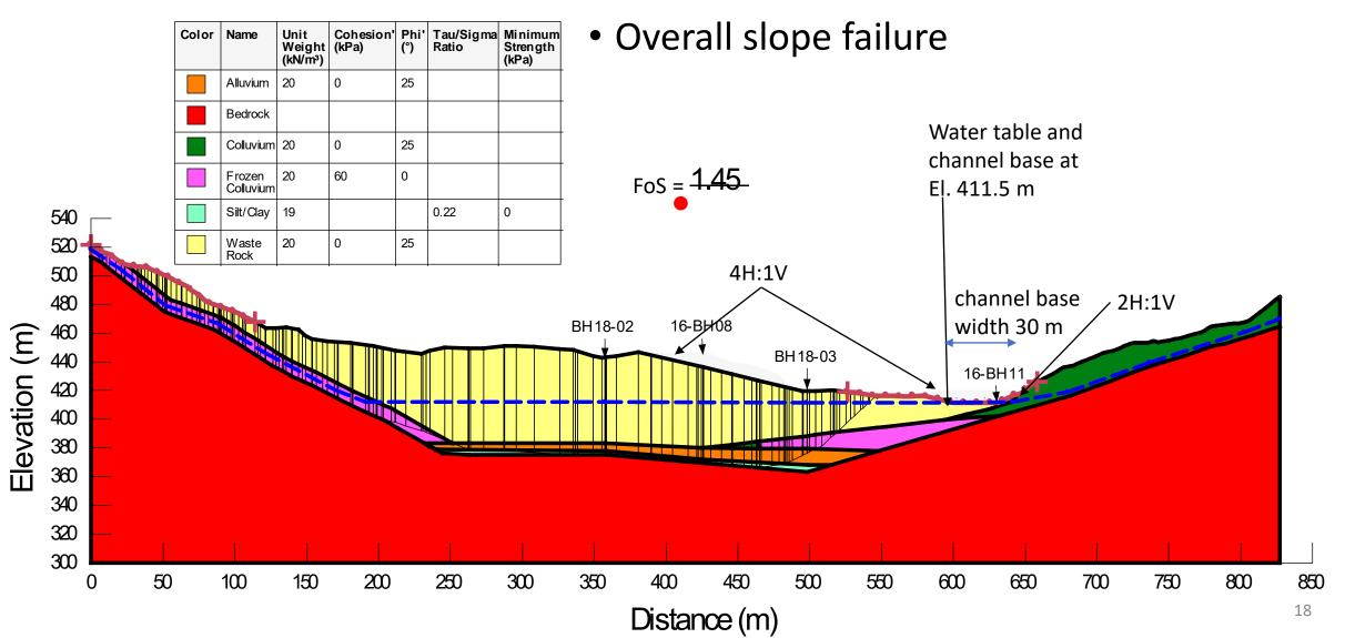
Option CC1 - Lake at El. 412 m Spillway Design Construction – Static liquefaction 4H:1V south side Spillway Channel slope
