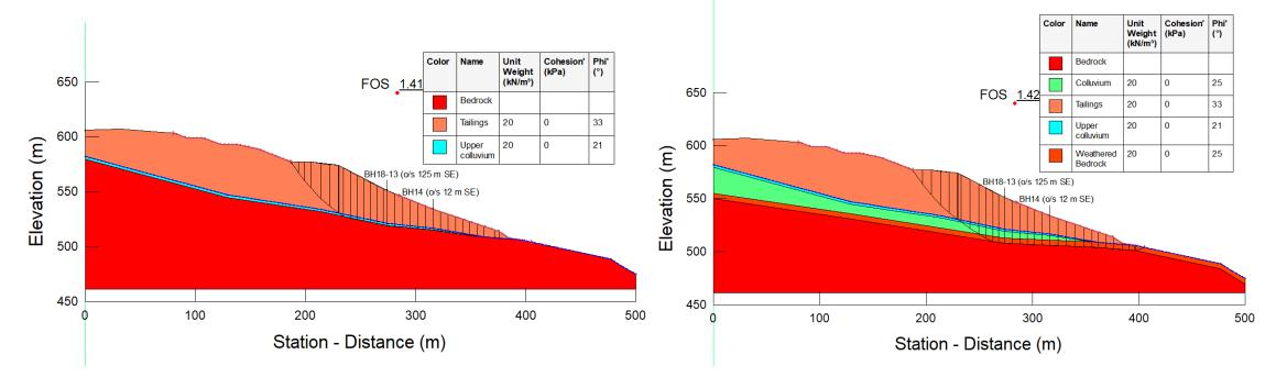
Without consideration of liquefaction, this cross-section has a FoS>1.3 for the current configuration.
