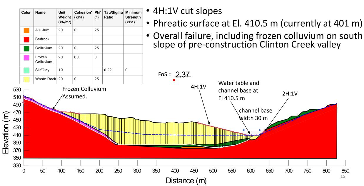
Scenario CC1 - Lake at El. 412 m Spillway Design Construction – Static liquefaction 4H:1V South Side Spillway Channel Slope
