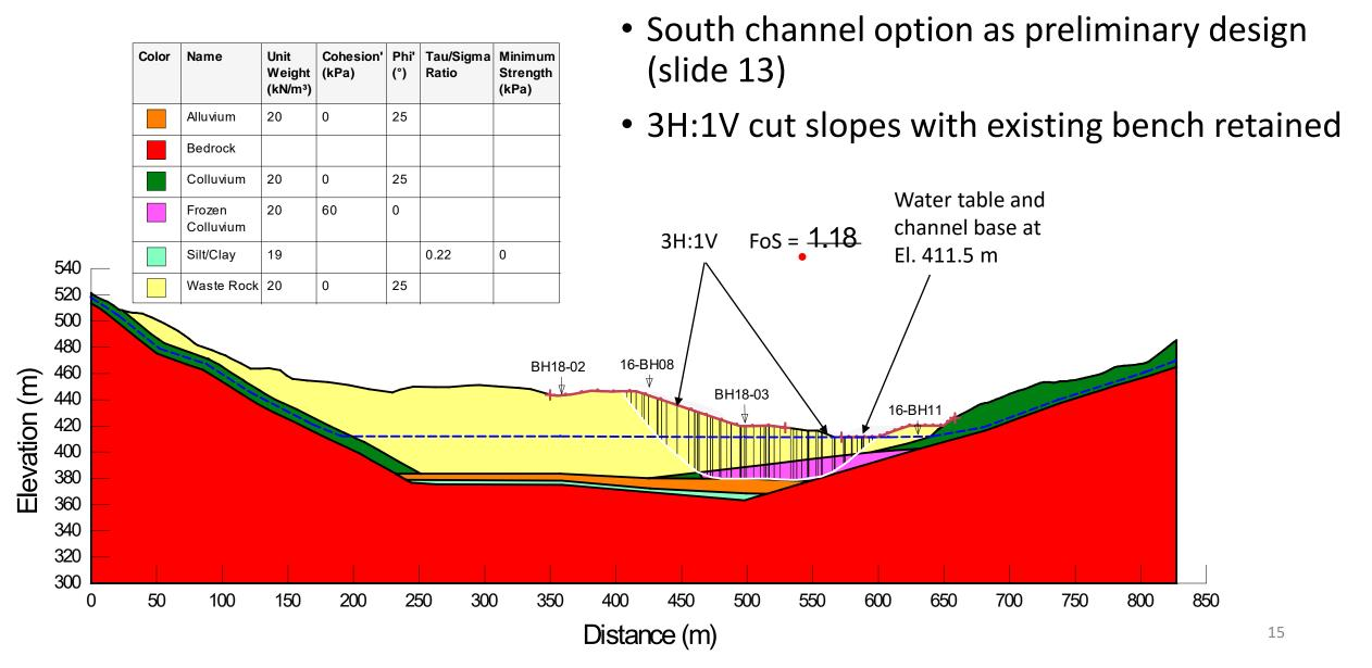
CC1 - DS4 Stability, South Channel Option, No Liquefaction 4H:1V slope cut, and Channel Base El. 411.5, width of ~32 m
