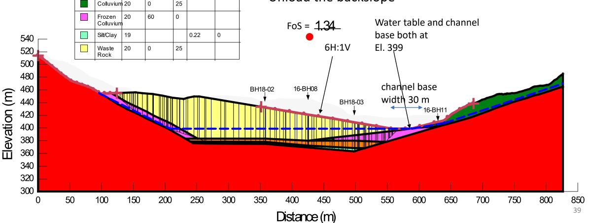
Option CC2 - Lake at El. 400 m Spillway Design Construction – Static liquefaction
