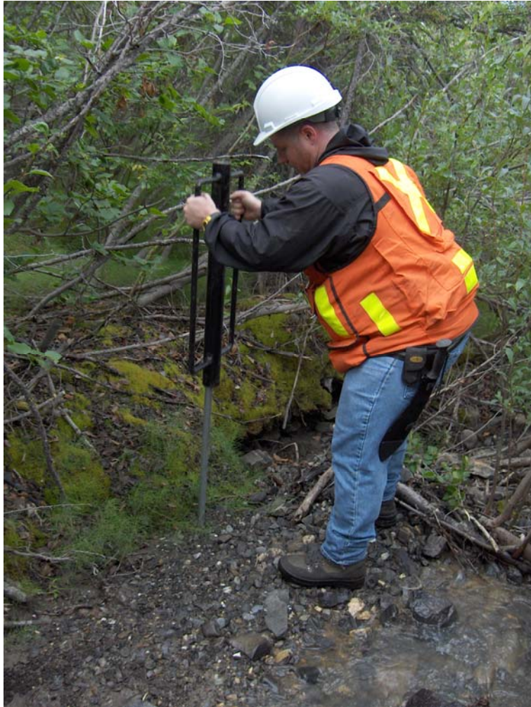
Photo 3: Access employee installing drivepoint piezometer
