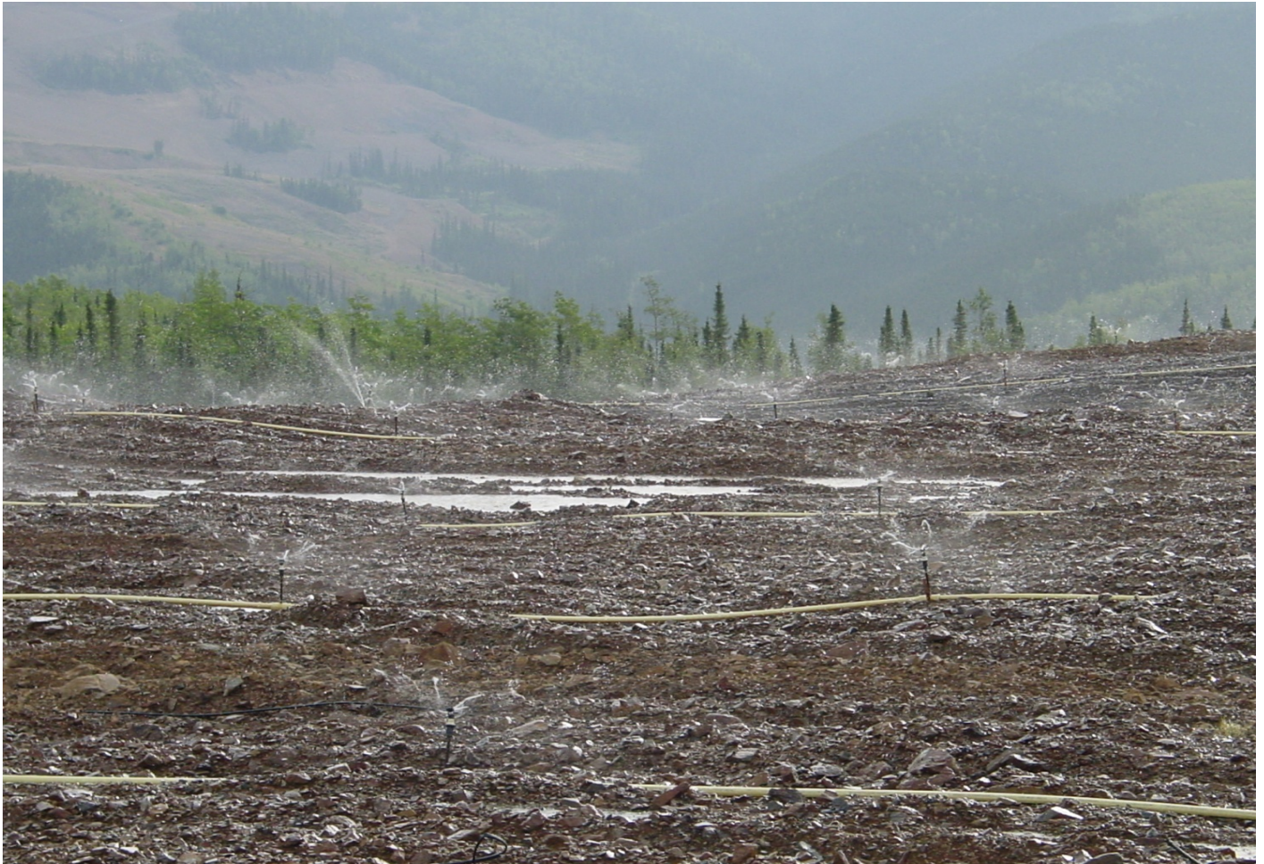
FIGURE 6. EXAMPLE OF HEAP LEACH (BREWERY CREEK MINE, YUKON)
