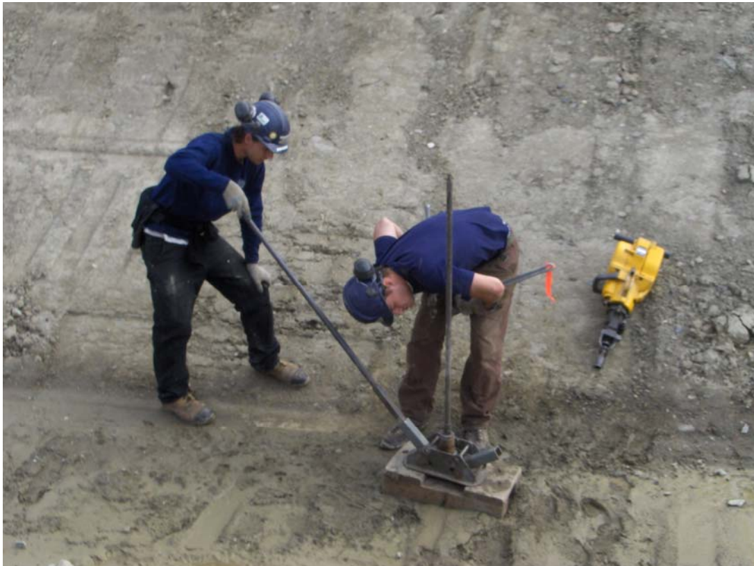
Photo 6: Sample Extraction technique
