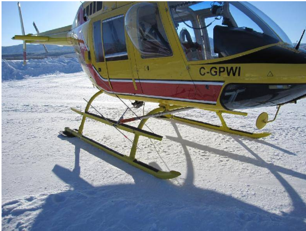
Photo 8. Telemetry H-antenna set-up for aerial surveys, February 12, 2014.
