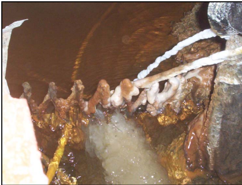
Plate 1 New lime slurry application point at weir in G300 adit.
