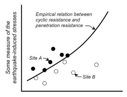
Some in situ test indice for liquefaction resistance
