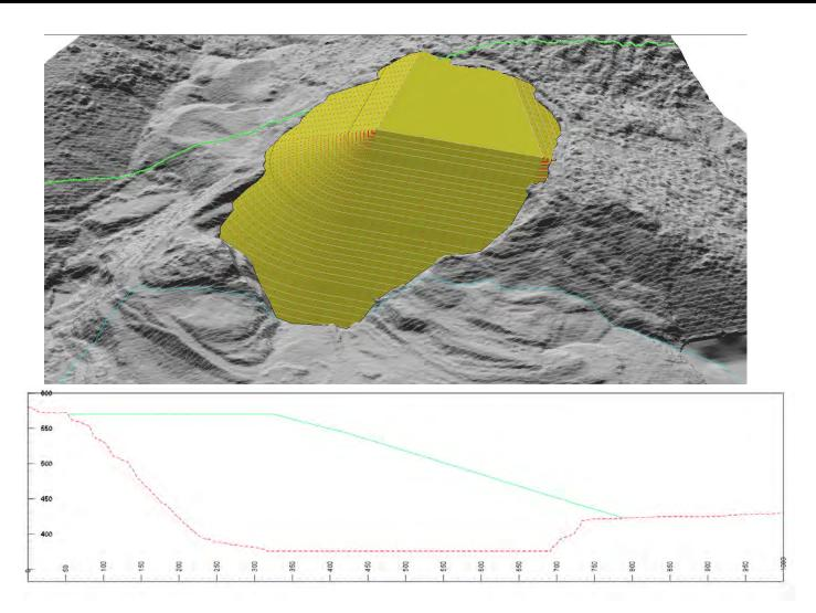
The overall storage capacity of the Porcupine Pit with assumed slopes of 3H:1V above the current topography, as shown, is approximatly  $23.9 \text{ M m}^3$ .
