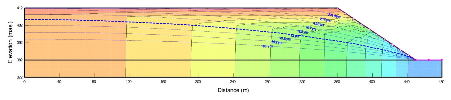
Figure 2: Predicted Drawdown vs. Time in Scenario 1a: Full Pit Drawdown (Ks = 1 x 10<sup>-6</sup> m/s for WRD and Basal Drain)
