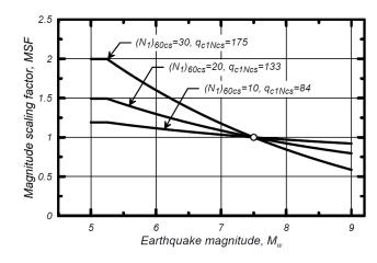
Figure 2.6. Variation in the MSF relationship with a large and with (N<sub>1</sub>)<sub>60x</sub> for cohesionless soils
