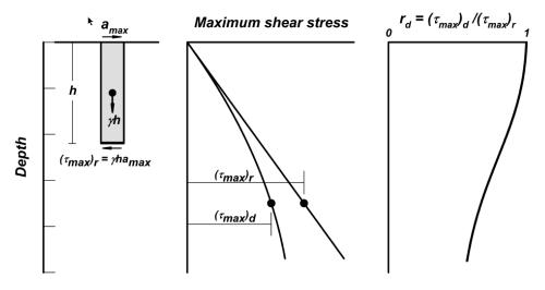
Figure 50. Schematic for determining maximum shear stress,  $\tau_{\text{max}}$ , and the stress reduction coefficient,  $r_d$ .
