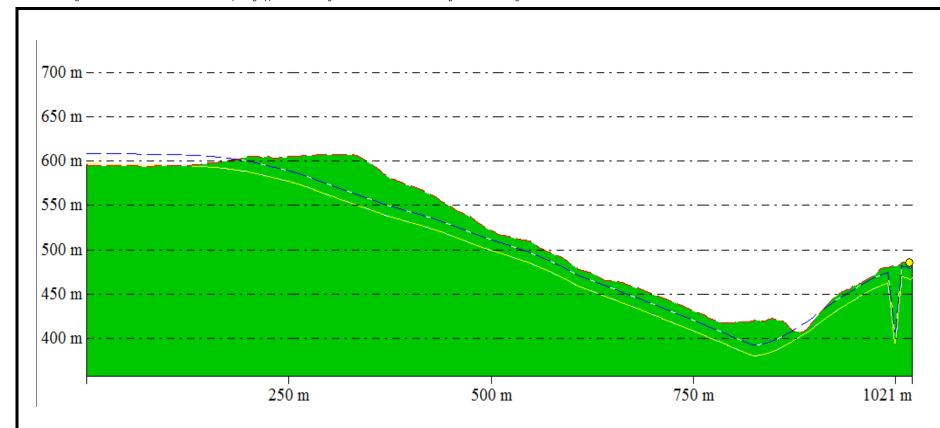
Cross-section of the south lobe of the Wolverine Tailings Dump, showing the 2012 DEM surface (the area colourd green), the 1949 DEM with the -13 m adjustment (blue dashed line) and the 1949 DEM with the -25 m adjustment (yellow line).
