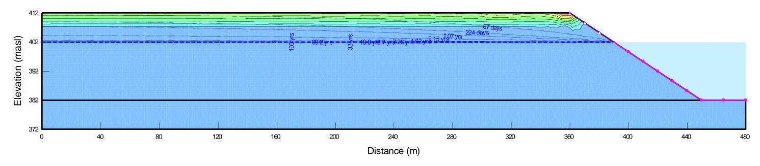
Figure 8: Predicted Drawdown vs. Time in Scenario 2b: 10m Pit Drawdown (Ks = 5 x 10<sup>-5</sup> m/s for WRD, 1 x 10<sup>-5</sup> m/s for Basal Drain)
