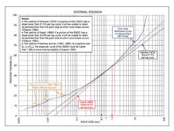
**Figure 6:** Evaluation the susceptibility to internal instability of the average grain size distribution curve corresponding to 25% fines using three different methods outlined in this memorandum.
