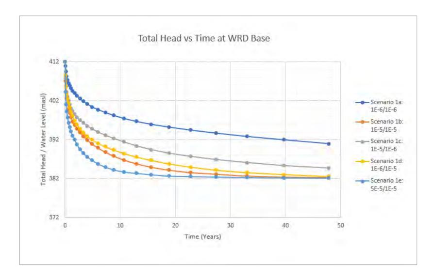
Figure 9: Predicted Total Head vs. Time at WRD Base in Scenario1 (a, b, c, d, e): Full Pit Drawdown (Note: values e.g. 5E-5/1E-5 in the legend stands for saturated hydraulic conductivities in m/s of WRD/Basal Drain)
