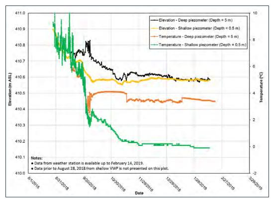
**Figure 4:** Plots of water level elevation vs time and temperature vs time from two piezometers installed on the lake shore relatively near the spillway since August 2018.
