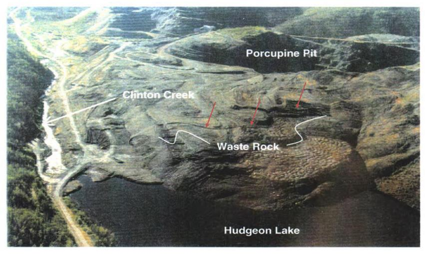
View of the Clinton Creek Waste Rock Dump facing east. Red arrows show the location of visible cracking indicating the extent of the slope failure.
