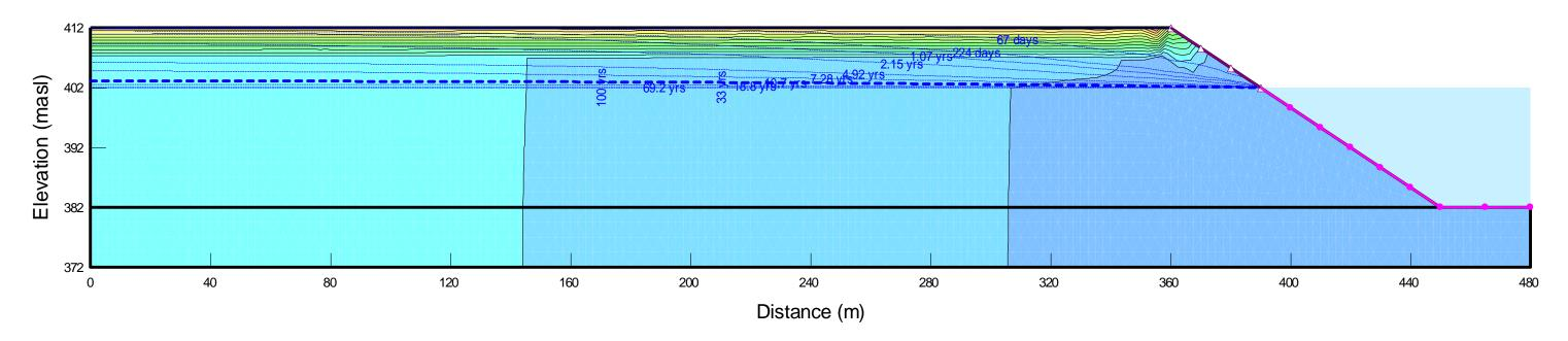
Figure 7: Predicted Drawdown vs. Time in Scenario 2a: 10m Pit Drawdown (Ks = 1 x 10<sup>-5</sup> m/s for WRD and Basal Drain)
