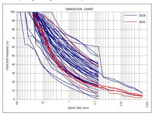
**Figure 1:** Grain-size distribution curves from 2016 and 2018 site investigation programs in the Clinton Creek Waste Rock dump.
