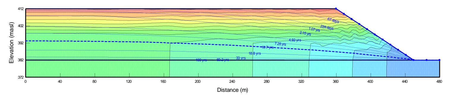
Figure 3: Predicted Drawdown vs. Time in Scenario 1b: Full Pit Drawdown (Ks =  $1 \times 10^{-5}$  m/s for WRD and Basal Drain)
