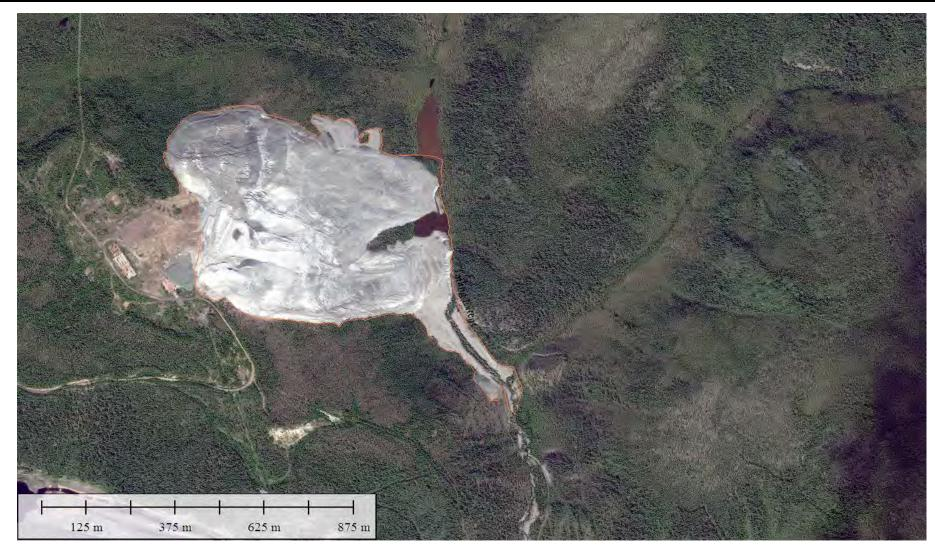
Plan view of the Wolvering Tailings Dump footprint, with a disturbed footprint of 448,000 m<sup>2</sup>.
