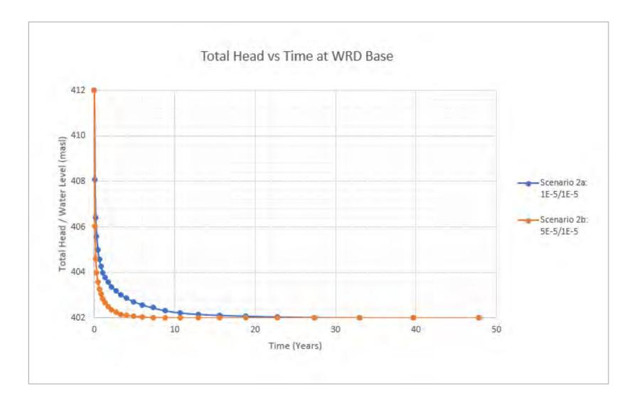
Figure 10: Predicted Total Head vs. Time at WRD Base in Scenario 2 (a, b): 10m Pit Drawdown (Note: values e.g. 5E-5/1E-5 in the legend stands for saturated hydraulic conductivities in m/s of WRD/Basal Drain)
