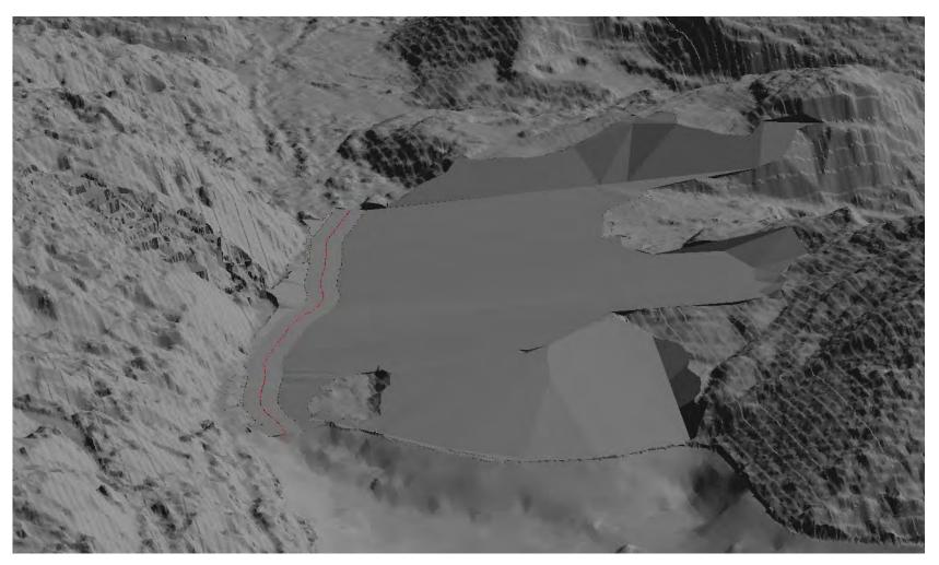
3-D model of the completed Clinton Creek Option 1 channel and excavated slopes, looking east
