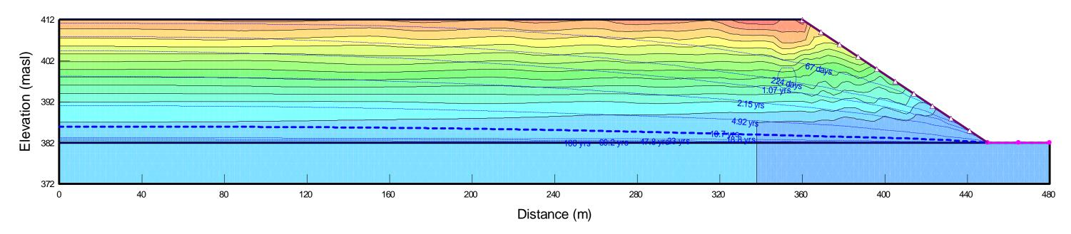
Figure 6: Predicted Drawdown vs. Time in Scenario 1e: Full Pit Drawdown (Ks = 5 x 10<sup>-5</sup> m/s for WRD, 1 x 10<sup>-5</sup> m/s for Basal Drain)
