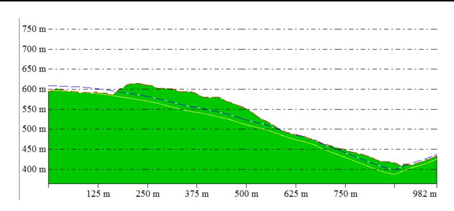
Cross-section of the north lobe of the Wolverine Tailings Dump, showing the 2012 DEM surface (the area colourd green), the 1949 DEM with the -13 m adjustment (blue dashed line) and the 1949 DEM with the -25 m adjustment (yellow line).
