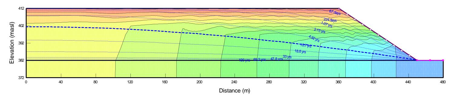
Figure 5: Predicted Drawdown vs. Time in Scenario 1d: Full Pit Drawdown (Ks = 1 x 10<sup>-6</sup> m/s for WRD, 1 x 10<sup>-5</sup> m/s for Basal Drain)
