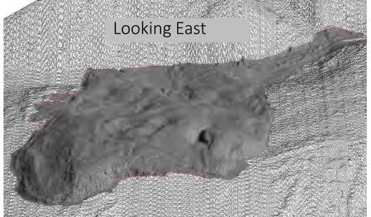
Plan View - Buttress fill at 4.5H:1V slope (E-W direction), side slopes of 3H:1 at north side, and various side slopes from 3H:1 (East) to 7H:1V (West) at the south side.
