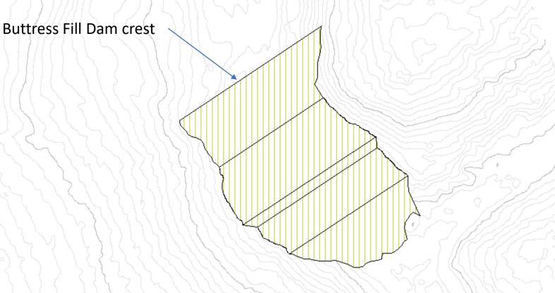
Volume of sub excavation (-7 m with side slope of 2H:1V) = 169,000 m<sup>3</sup>
