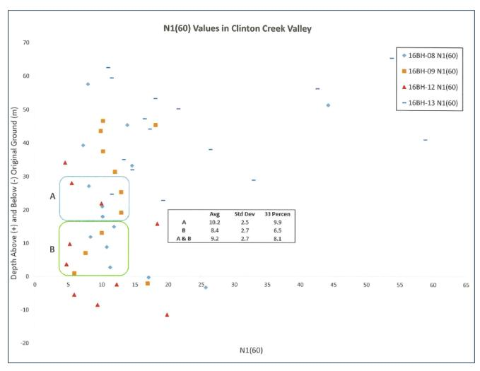
Figure 2: SPT Data for Clinton Creek Valley Waste Landside Dam Waste Dumps
