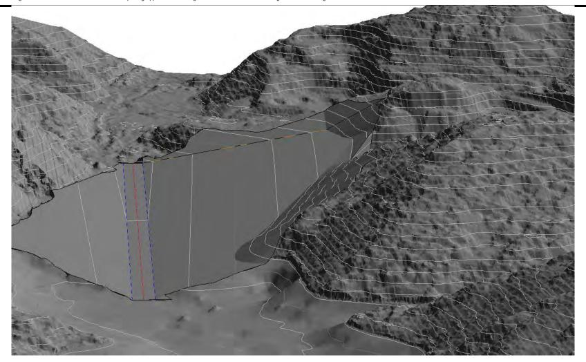
3-D model of the completed Clinton Creek Option 3 channel and excavated slopes, looking east
