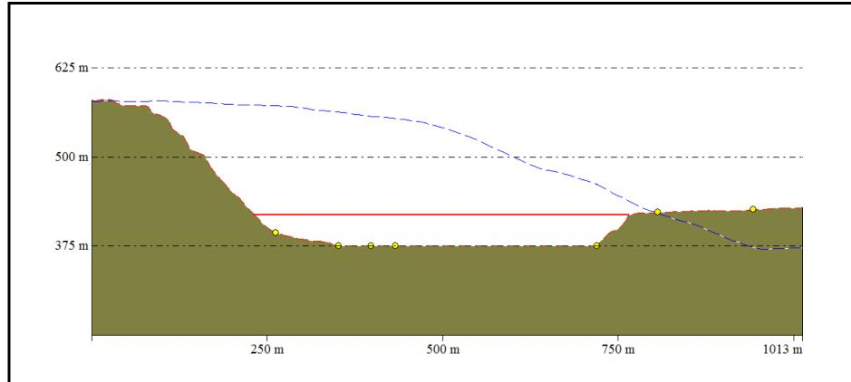
Estimated volume available for fill placement between El. 375 m (top of the Porcupine Pit Lake) and the north rim of the Porcupine Pit at El. 418 m (shown by the red line in the cross-section) is 2.6 M m3
