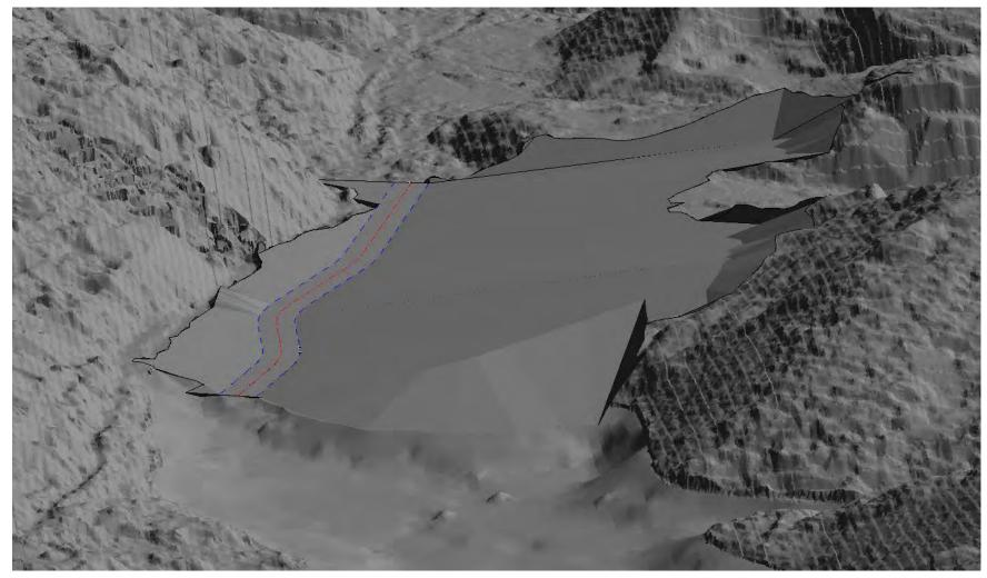
3-D model of the completed Clinton Creek Option 2 channel and excavated slopes, looking east
