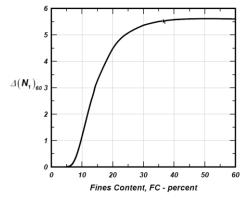
Fines content 30% correction  $\Delta N = 5.5$ ; N1(60)CS =8+5.5 = 13.5 Fines 15%,  $\Delta N = 3$ : N1(60)CS = 5+3 = 8
