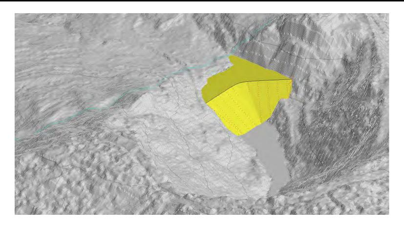
The initial shell required along the north pit wall of Porcupine Pit, with a slope of 2H:1V up to the lip of the pit at El. 418 m.
