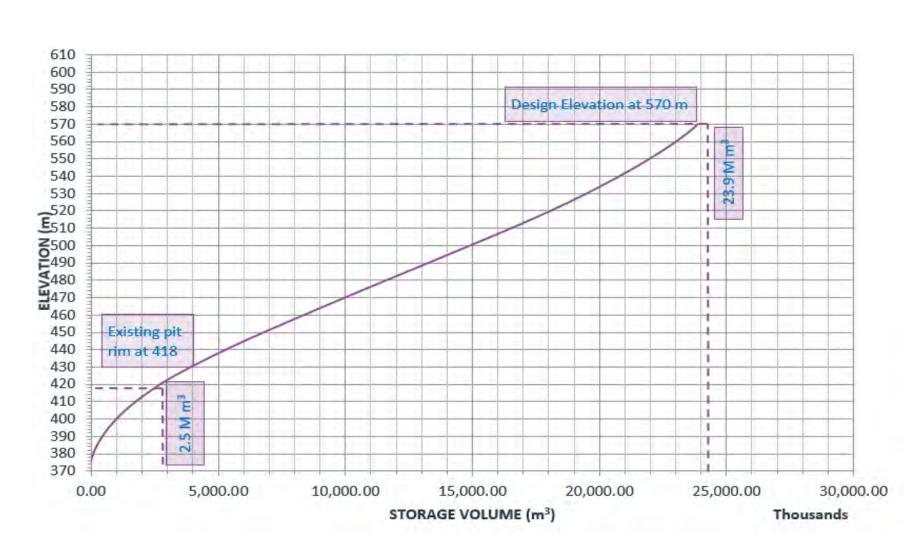
The overall storage capacity of the Porcupine Pit with assumed slopes of 3H:1V above the current topography, as shown, is approximatly 23.9 M m<sup>3</sup>.
