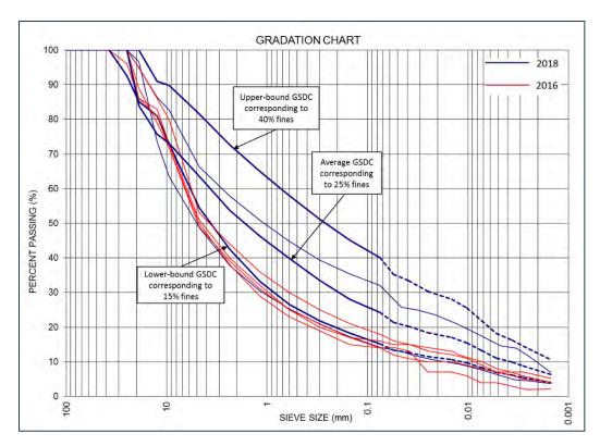
**Figure 2:** Selected complete grain-size distribution curves (sieving and sedimentation) used in the hydraulic conductivity calculations.
