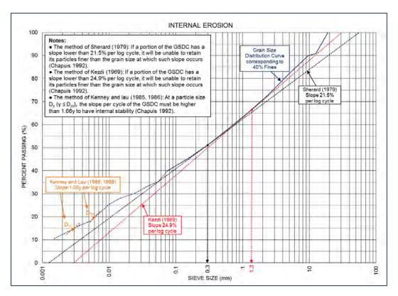
**Figure 5:** Evaluation the susceptibility to internal instability of the upper-bound grain size distribution curve corresponding to 40% fines using three different methods outlined in this memorandum.
