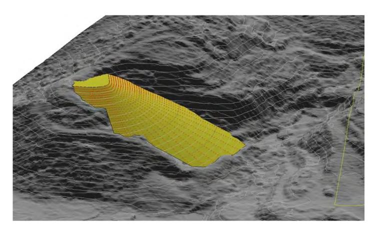
The estimaged potential storage volume available in the Snowshoe Pit is  $608,000 \, \text{m}^3$ , based on the assumed 3H:1V slopes shown.
