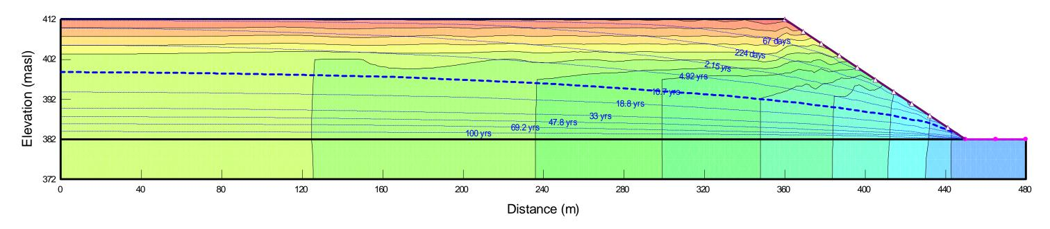
Figure 4: Predicted Drawdown vs. Time in Scenario 1c: Full Pit Drawdown (Ks = 1 x 10<sup>-5</sup> m/s for WRD, 1 x 10<sup>-6</sup> m/s for Basal Drain)
