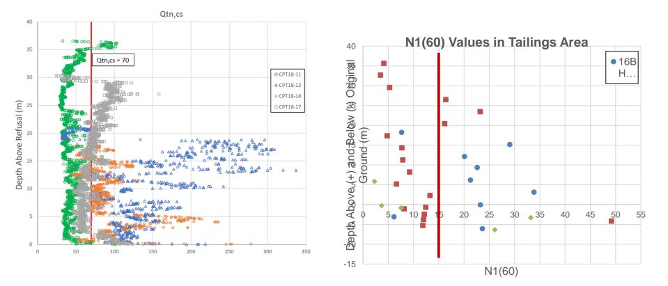
Both SPT N1(60) and CPT qtn,cs data are available for the tailings. Sand state Qtn,cs = 70 and N1(60) are considered susceptible liquefaction. Consistently loose tailings is found in the upper slope, versus higher indicated state in the lower slope.
