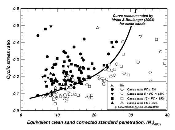
Figure 75. SPT case histories of liquefaction in cohesionless soils with various fines contents plotted versus their equivalent clean sand  $(N_1)_{60cs}$  values for M = 7.5 and  $\sigma'_{vc}$  = 1 atm.
