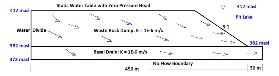
Figure 1: Conceptual Groundwater Flow System
