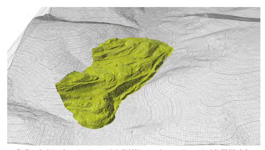
The Clinton Creek Waste Dump, shown in green with the 2012 DEM contours shown, contains approximatly 21,657,000 m3 of waste material, based on the difference between the 2012 DEM and the 1949 DEM.
