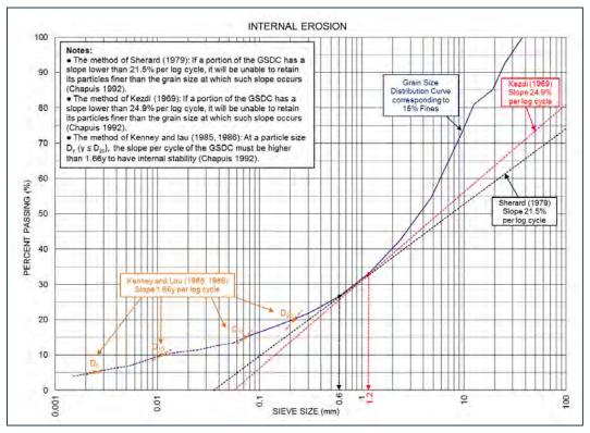
**Figure 7:** Evaluation the susceptibility to internal instability of the lower-bound grain size distribution curve corresponding to 15% fines using three different methods outlined in this memorandum.
