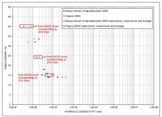
Figure 3: Hydraulic Conductivity vs Fines Content from the Clinton Creek Waste Rock Dump.
