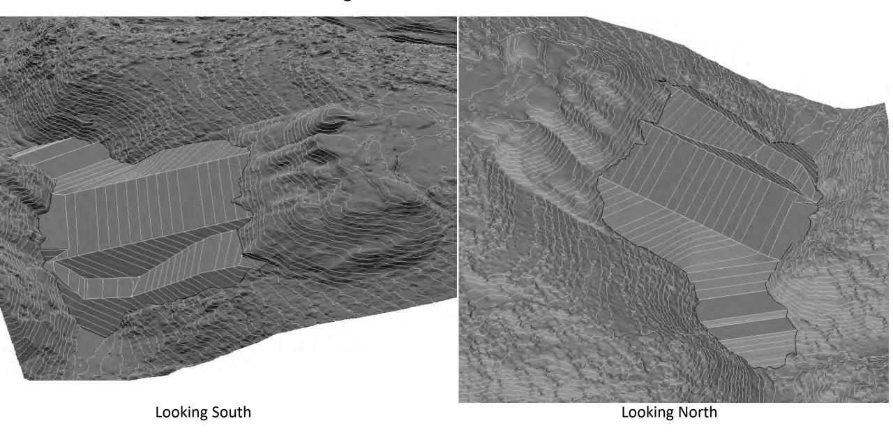
Total Fill volume = 5,150,000 m<sup>3</sup> including filters, and excluding sub excavation <sup>14</sup>
