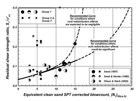
Figure 89. Normalized residual shear strength ratio of liquefied sand versus equivalent clean-sand SPT-corrected blow count for  $\sigma'_{vc} < 400$  kPa, using the case histories published by Seed (1987), Seed and Harder (1990), and Olson and Stark (2002).
