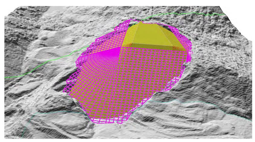
The final shell design to El. 570 m with a 3H:1V slope between El. 418 and El. 570 m
