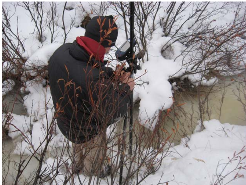
Photograph 8. Surveying Pony Creek to obtain a stream profile.
