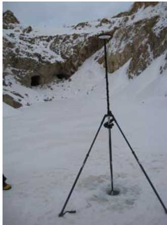
Photograph 9. Surveying pit lake water elevation and pit water sampling location; adits located in background.
