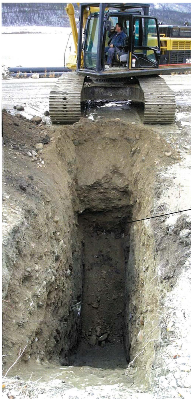
Photo I-11 TPKC07-3 exposed 3.5 m of fill, with sand and gravel underlying to at least 5.5 m depth. Note the thin black buried soil layer at 3.5 m depth.
