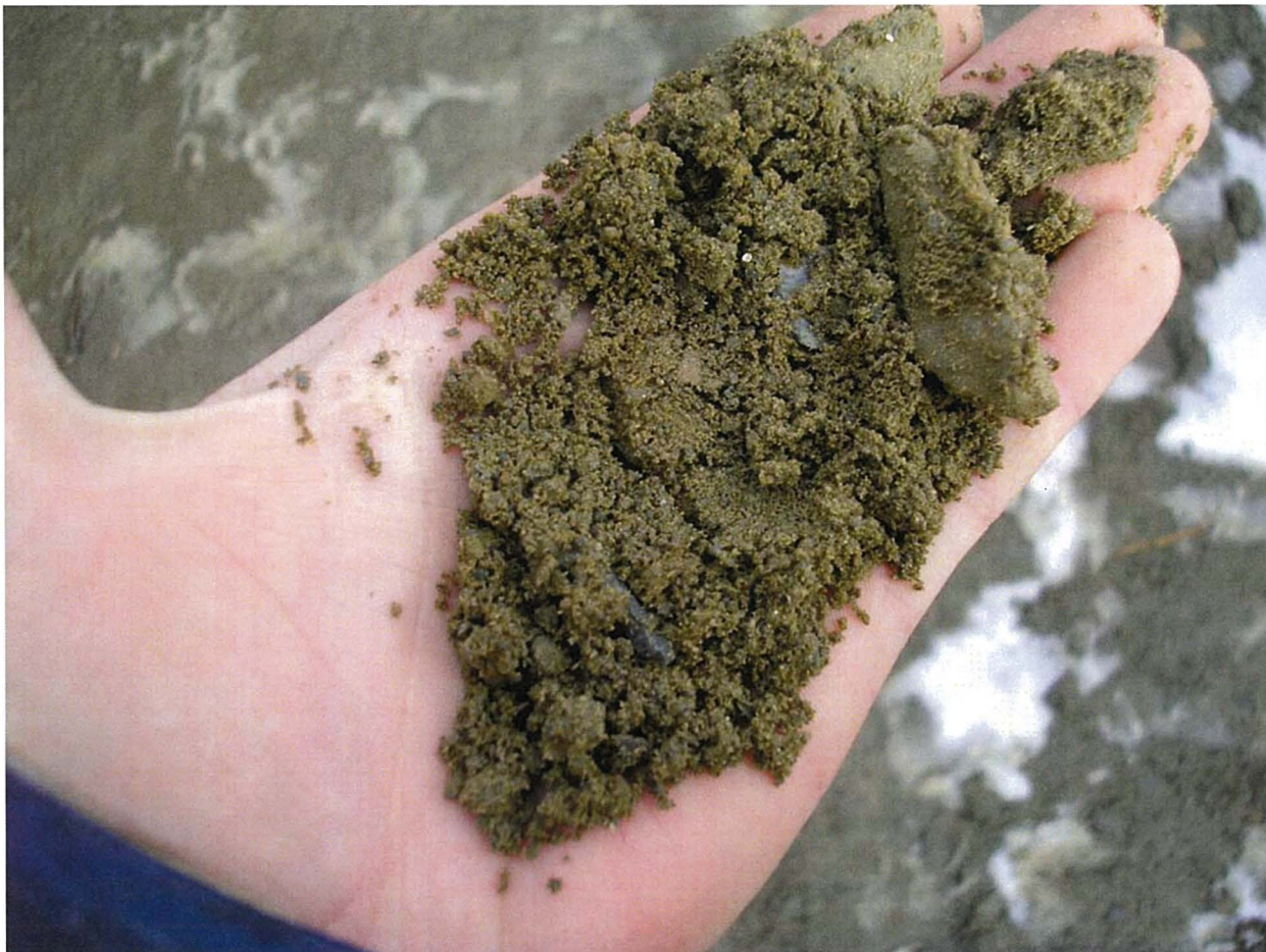
Photo I-3 Sand and gravel chip sample from tri-cone drilling at about 4 m depth at DHKC07-1.
