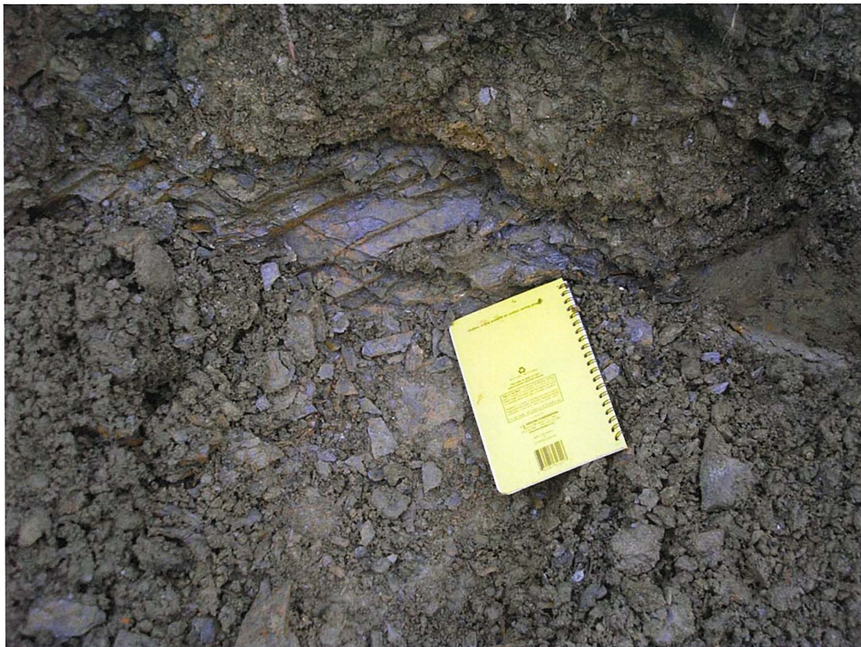
Photo I-5 Foliated schist bedrock in a dozer cut at DHKC07-2.
