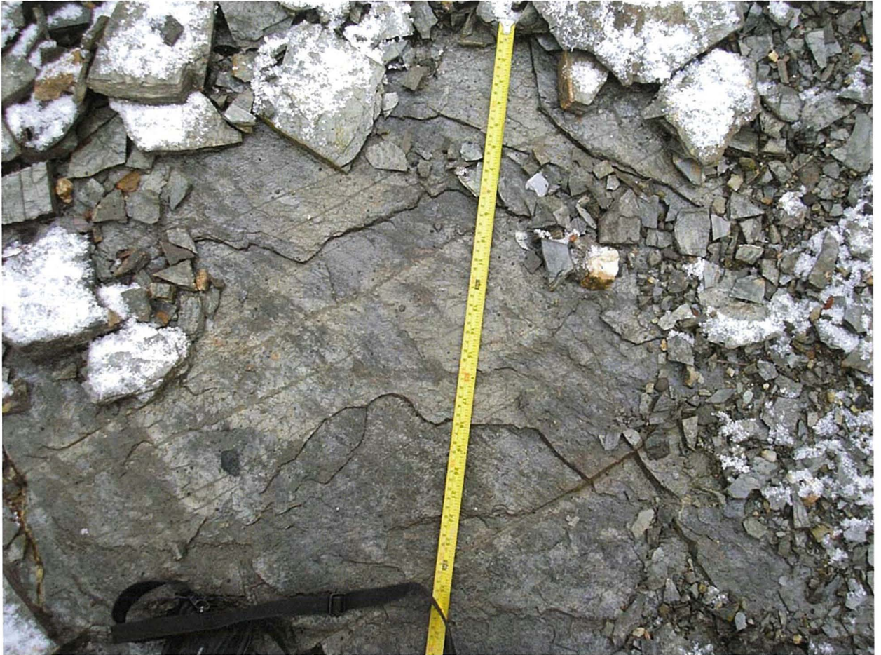
Photo I-13 The smooth, planar surface of foliation in the schist bedrock in a roadcut at 07SE28-1. Foliation spacing is 2 to 10 mm.
