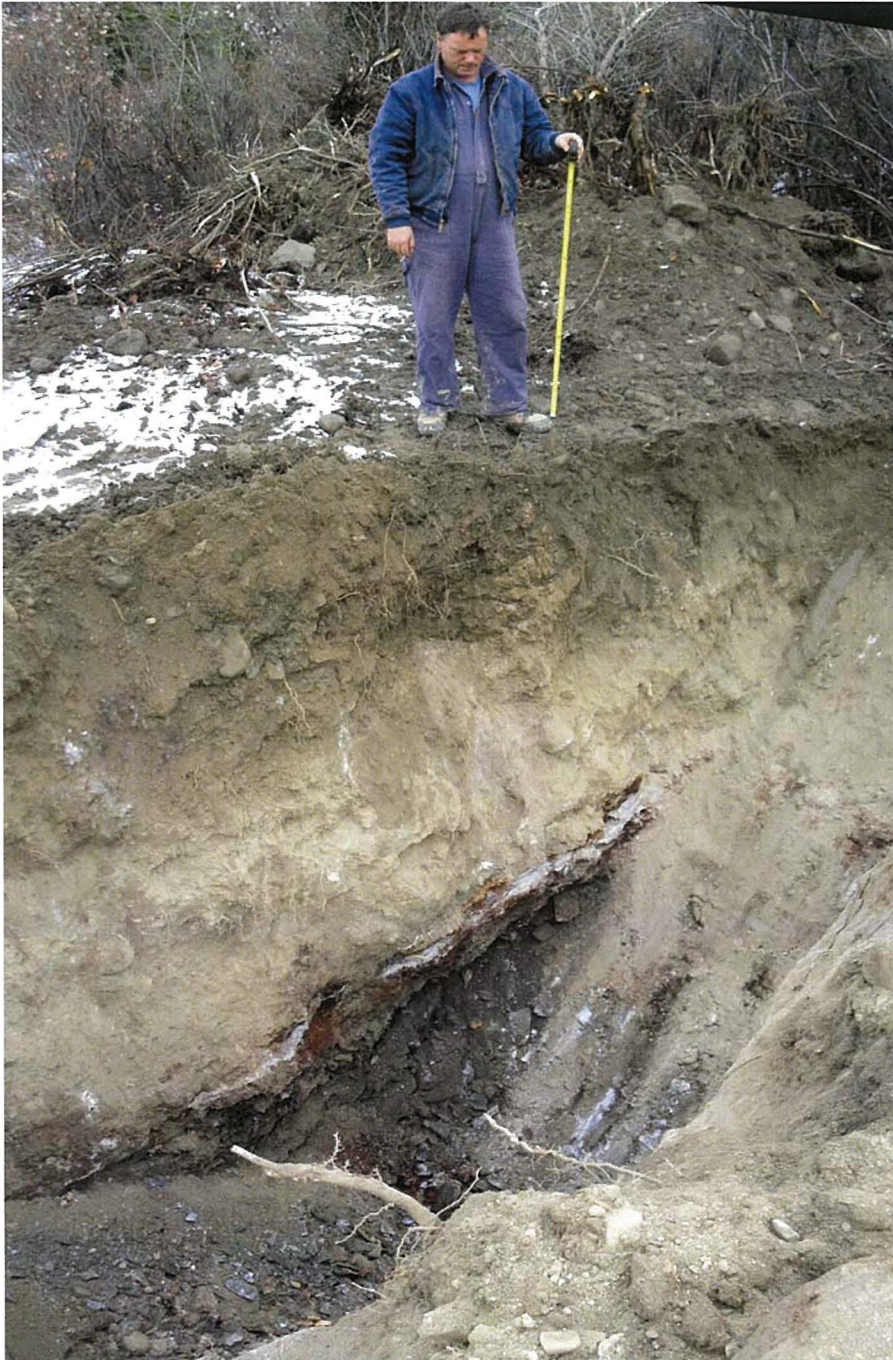
Photo I-10 TPKC07-2 exposed schist bedrock at 1.9 m below surface. Note the darker disturbed material at the top of the test pit.
