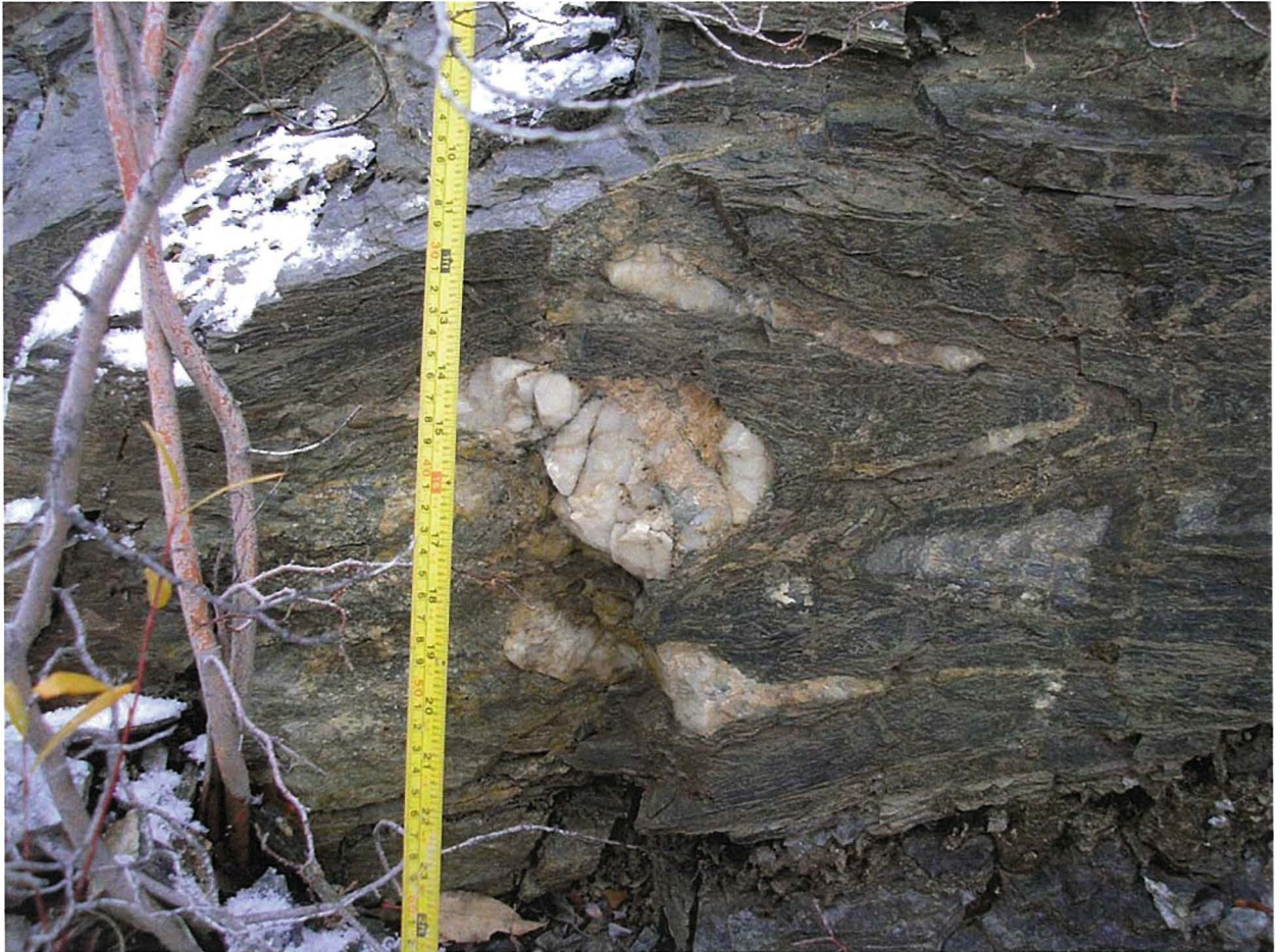
Photo I-14 Closely foliated schist with minor folding in a roadcut at 07SE28-1. The light material is quartz.
