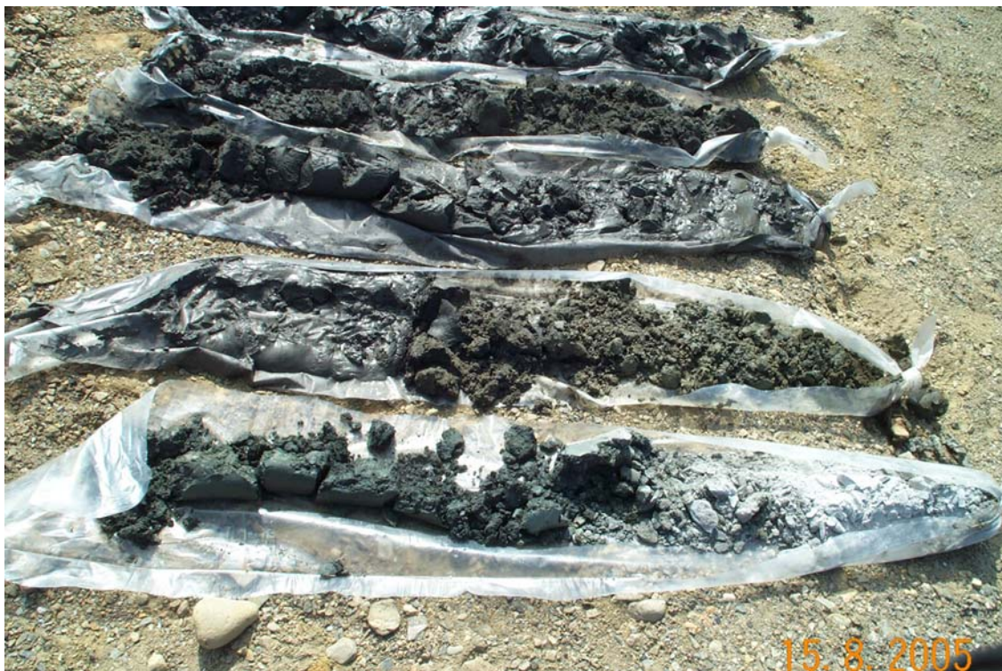
Photo of sample from ETA-05-3. Sample order is as indicated by upper photo, so the material from the bottom of the hole is at front right.
