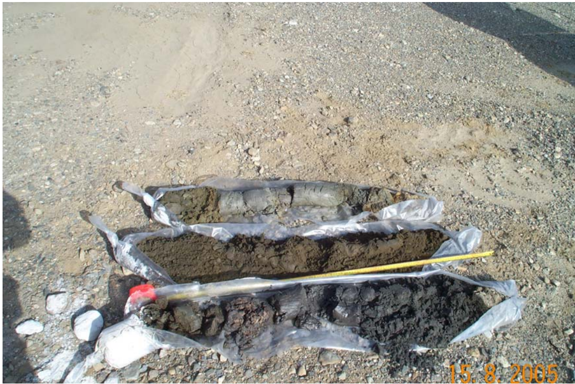
Photo of sample obtained with Sonic Drill from hole ETA-05-2. Material from top of hole is at left rear. Sample at depth is laid out sequentially left to right, back to front.
