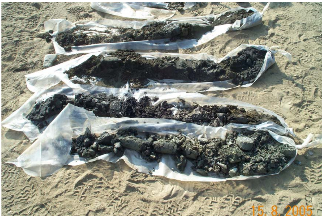
Photo of sample from ETA-05-5. Sample order is as indicated by upper photo, so the material from the bottom of the hole is at front right.
