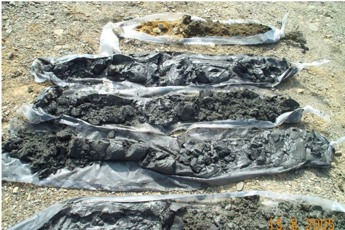
Photo of sample obtained with Sonic Drill from hole ETA-05-3. Material from top of hole is at left rear. Sample at depth is laid out sequentially left to right, back to front.
