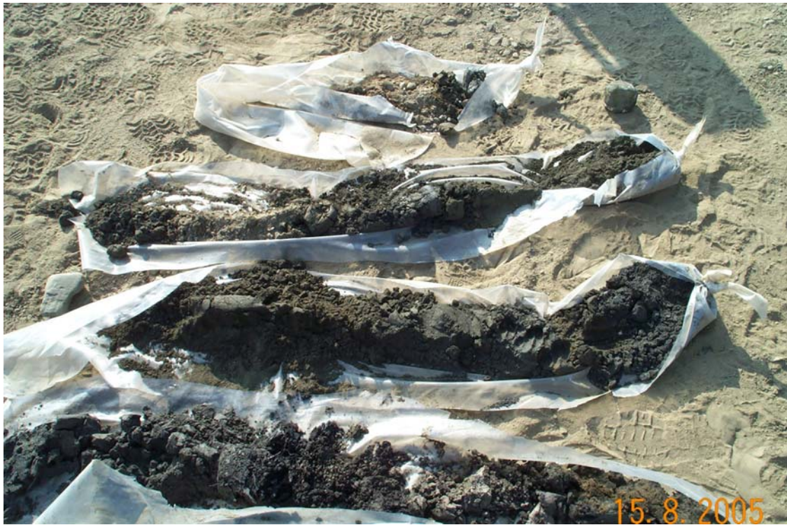
Photo of sample obtained with Sonic Drill from hole ETA-05-5. Material from top of hole is at left rear. Sample at depth is laid out sequentially left to right, back to front.
