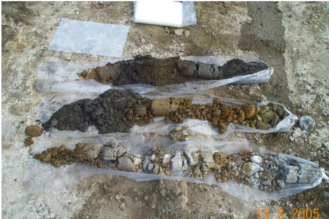
Photo of sample obtained with Sonic Drill from hole ETA-05-1. Material from top of hole is at left rear. Sample at depth is laid out sequentially left to right, back to front.
