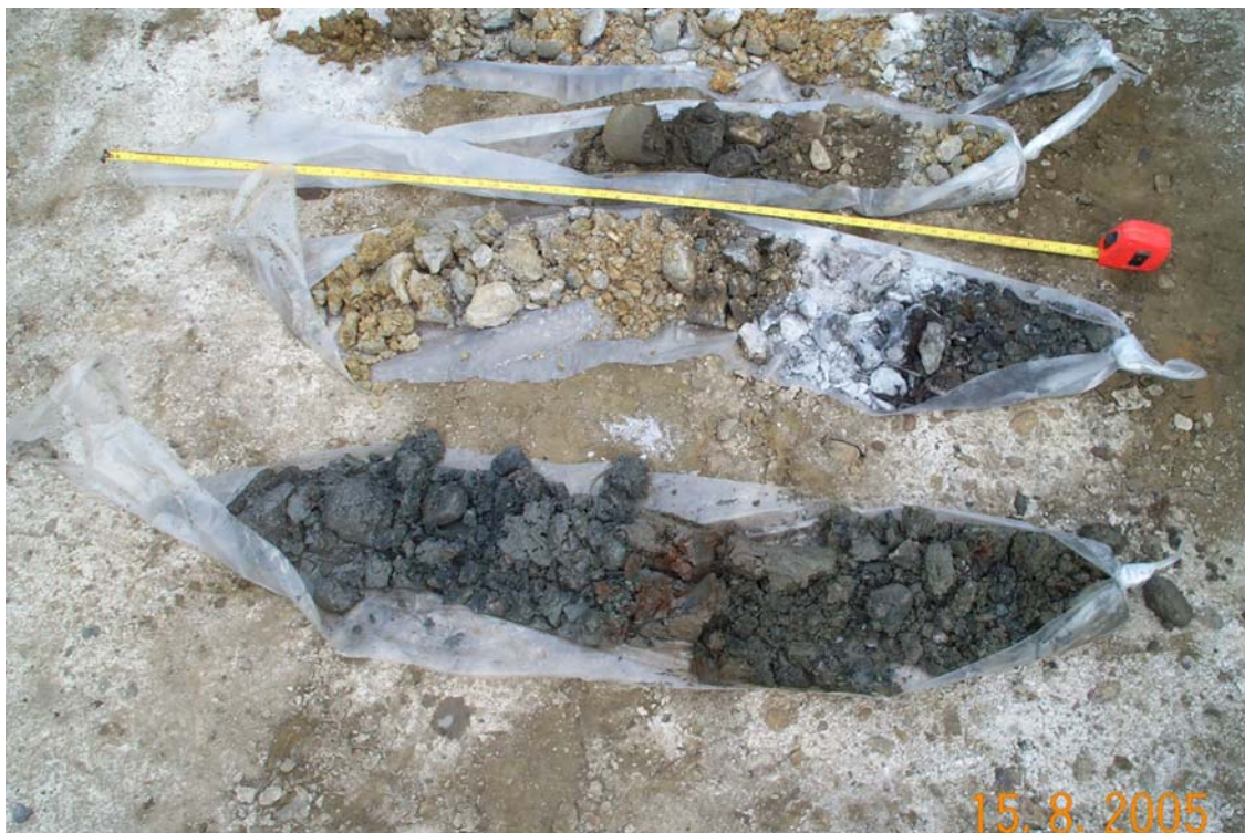
Photo of sample from ETA-05-1. Sample order is as indicated by upper photo, so the material from the bottom of the hole is at front right.
