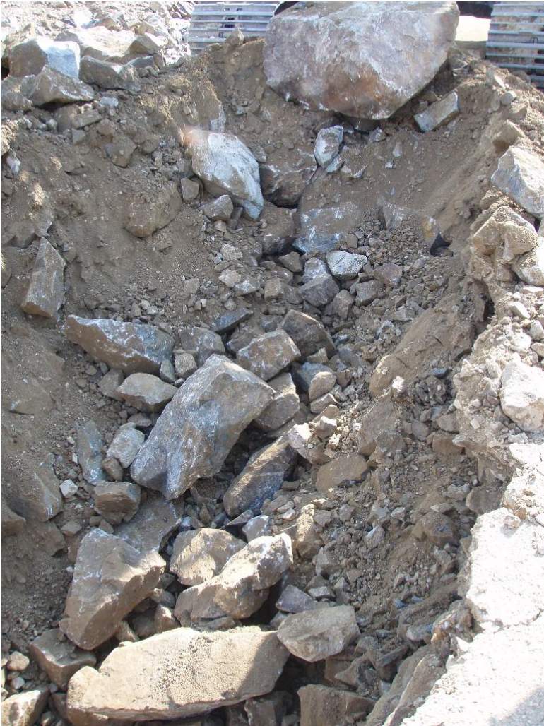
Photo 1. Test pit HR13, very blocky digging with minor amount of fines.
