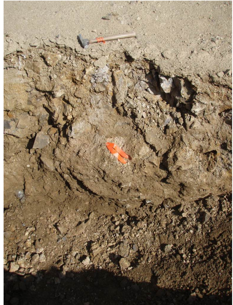
Photo2. Test pit HR20, typical of material backfilled in road bed.
