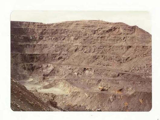
10. West wall of Porcupine Pit. Pit wall above El. 1380 bench (i.e. the bench above that on which loader is working) is final. Further excavation is planned below El. 1380, leaving a 58-ft. wide bench at El. 1380.
