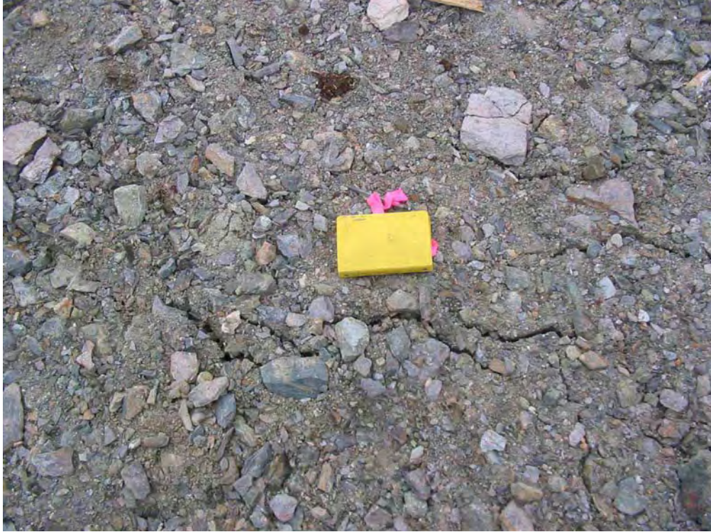
Figure 1. East test cover: Small cracks along eastern edge.
