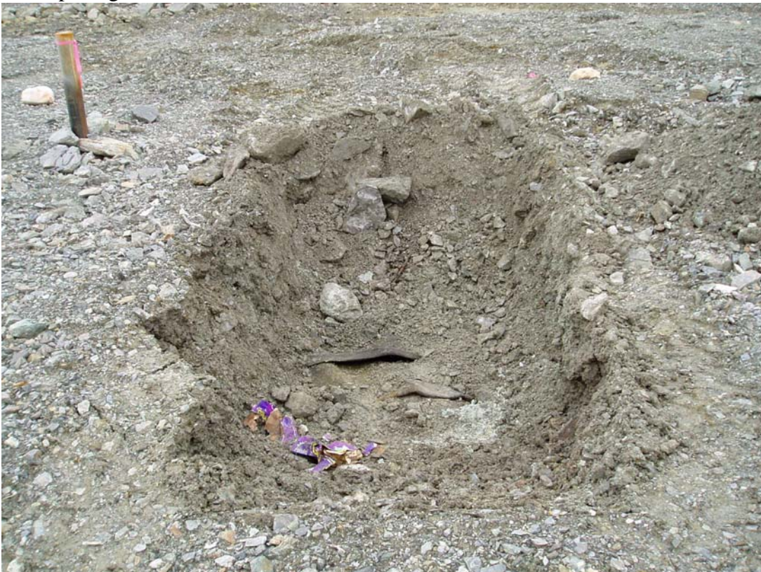
Photo 16: TP-TTC-04-05 Complete view of test pit showing gradation of the cover material.
