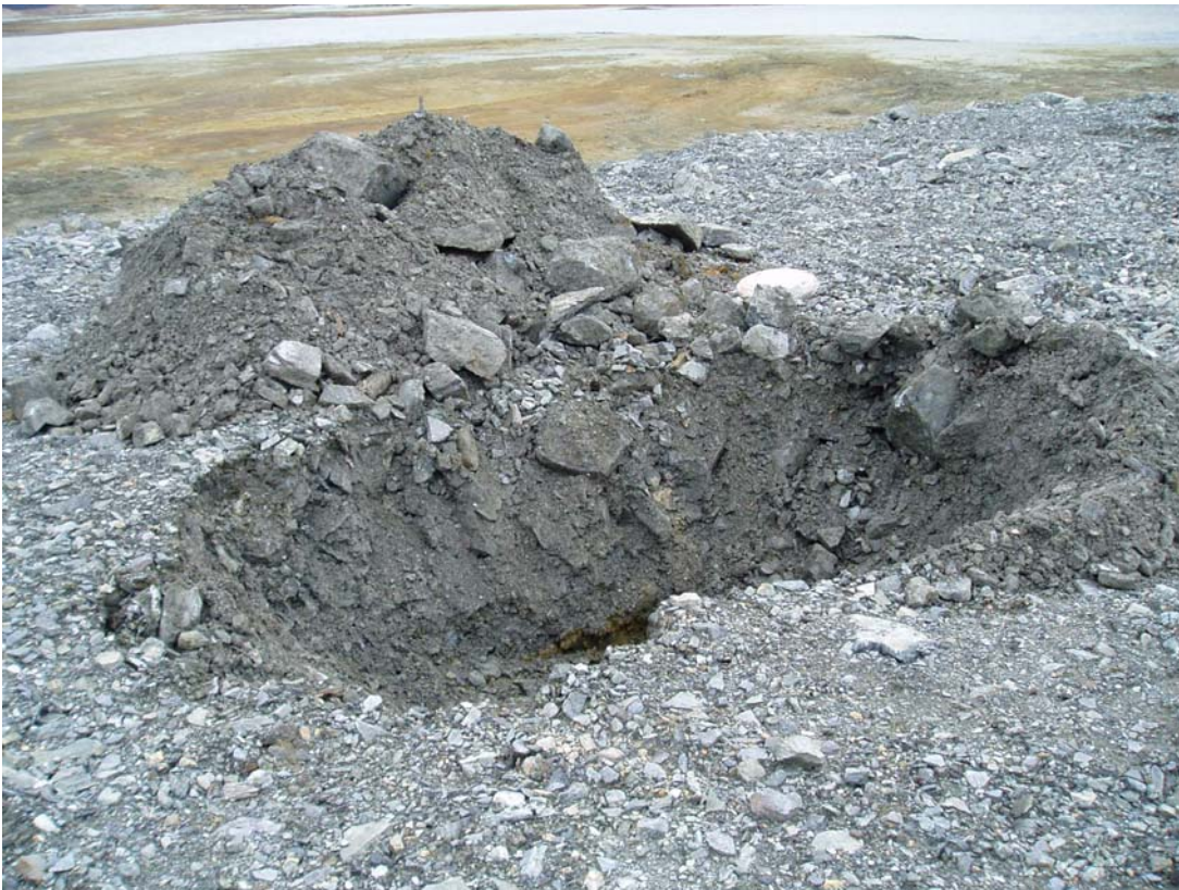
Photo 4: TP-TTC-04-01 View of complete test pit showing range in grain size from fines to boulders measuring 50 cm in diameter.
