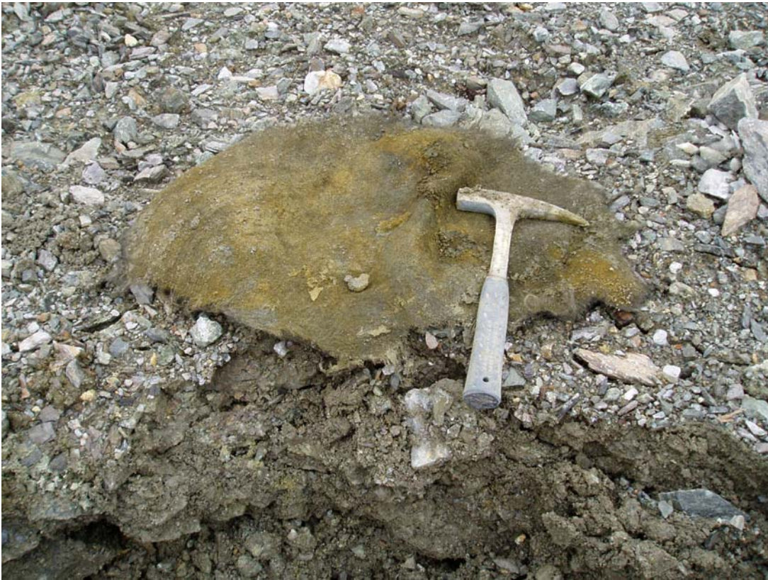
Photo 13: TP-TTC-04-04 The bottom of the geotextile is stained with tailings. It is possible that tailings is clogging the geotextile and subsequently slowing down the consolidation time.
