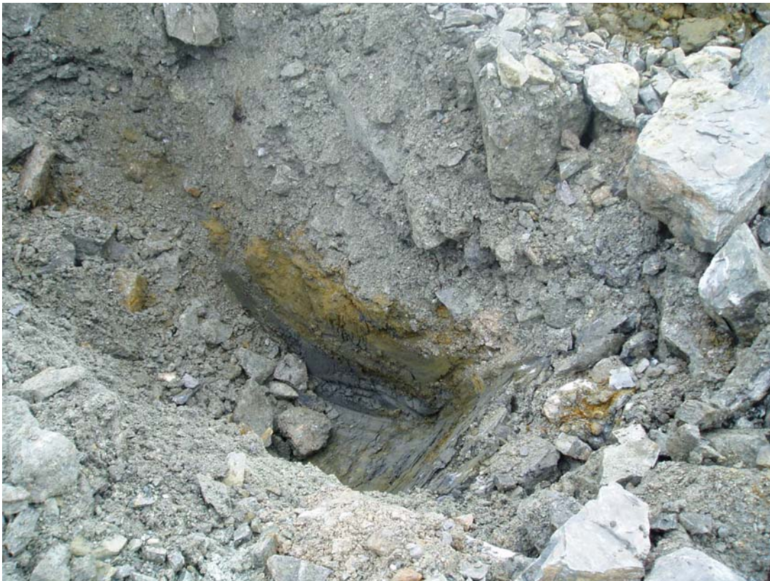
Photo 5: TP-TTC-05-02 Profile of test pit showing range of particle sizes in cover material.
