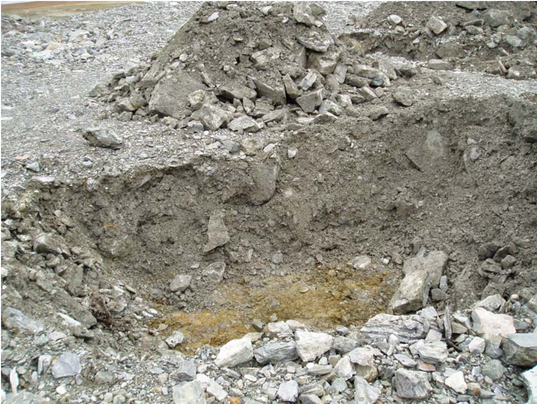
Photo 10: TP-TTC-04-03 Profile showing the range of particle sizes in the cover material.
