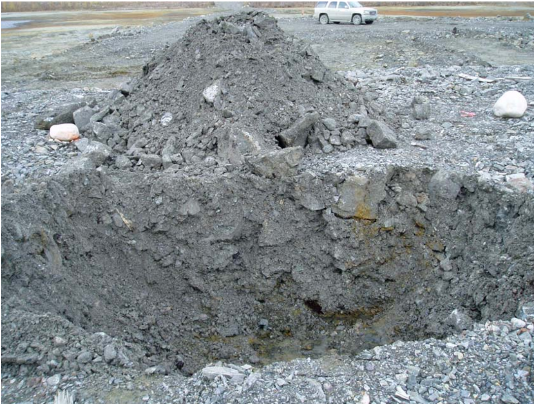
Photo 7: TP-TTC-04-02 Overall view of test pit showing range in grain size distribution of cover material.
