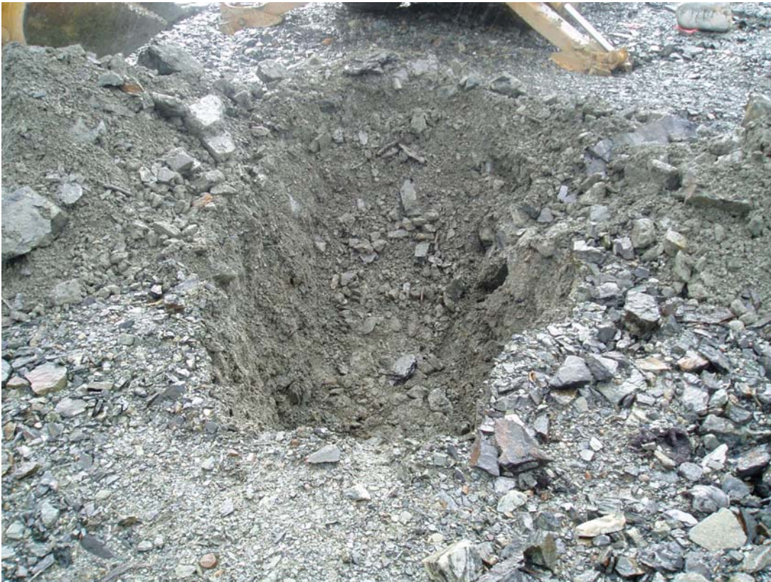
Photo 15: TP-TTC-05-06 Complete view of test pit showing gradation of the cover material.
