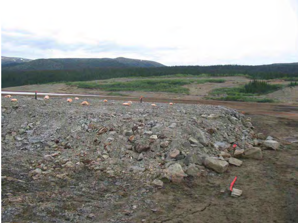
Figure 5. East test cover: Eastern edge, showing slightly undulating surface.
