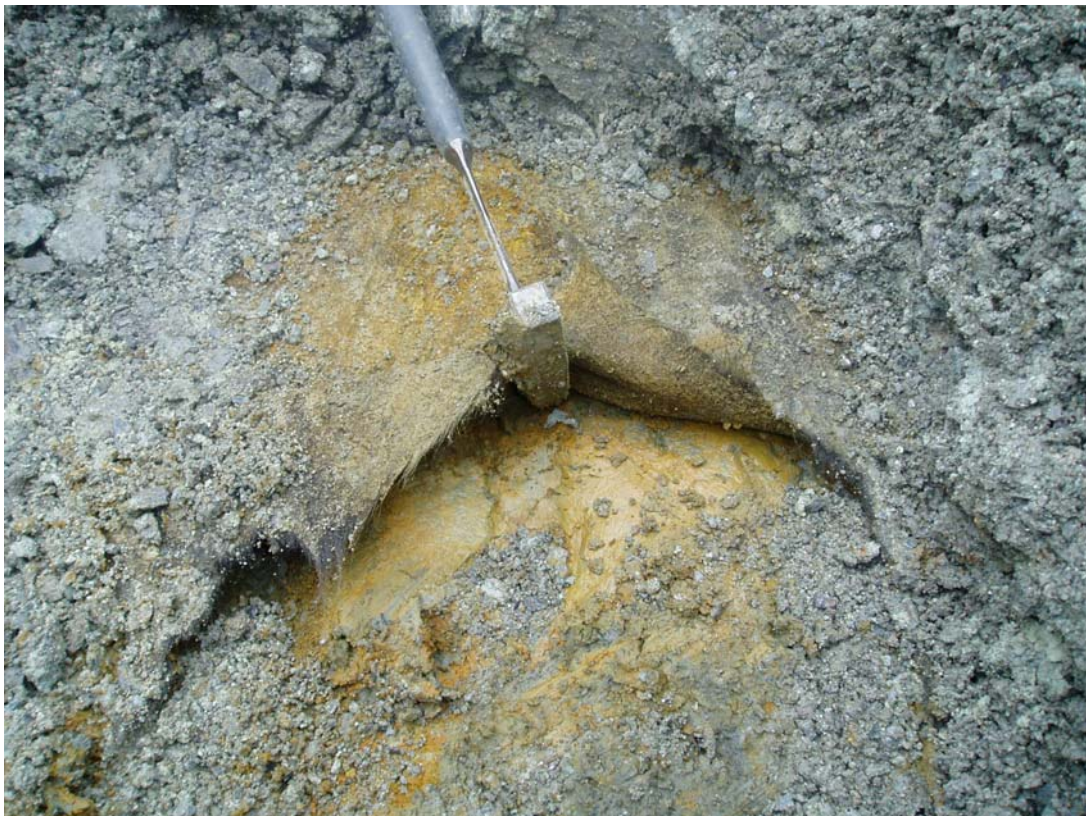
Photo 10: TP-TTC-05-04 Contact between cover material and tailings.
