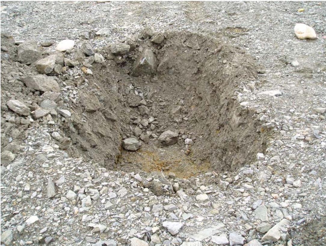
Photo 3: TP-TTC-04-01 View of complete test pit showing the range amount of fines present in the cover material.
