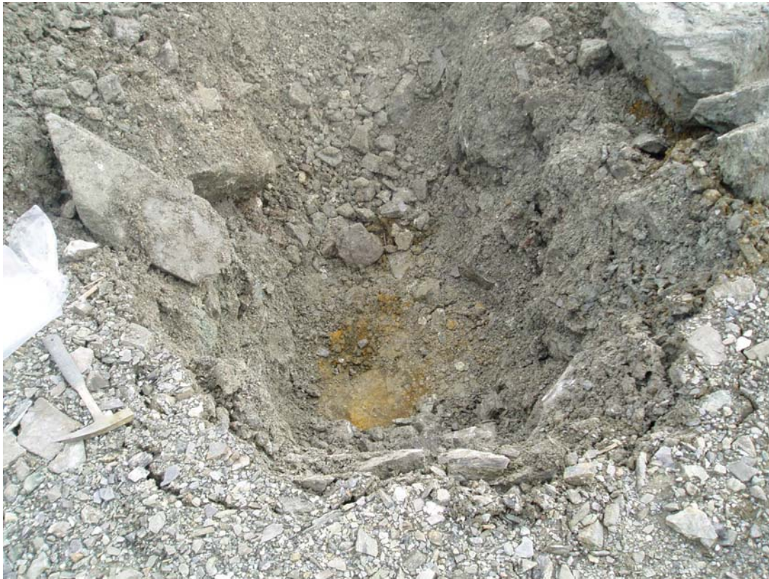
Photo 11: TP-TTC-05-04 The tailings has not migrated through the geotextile.
