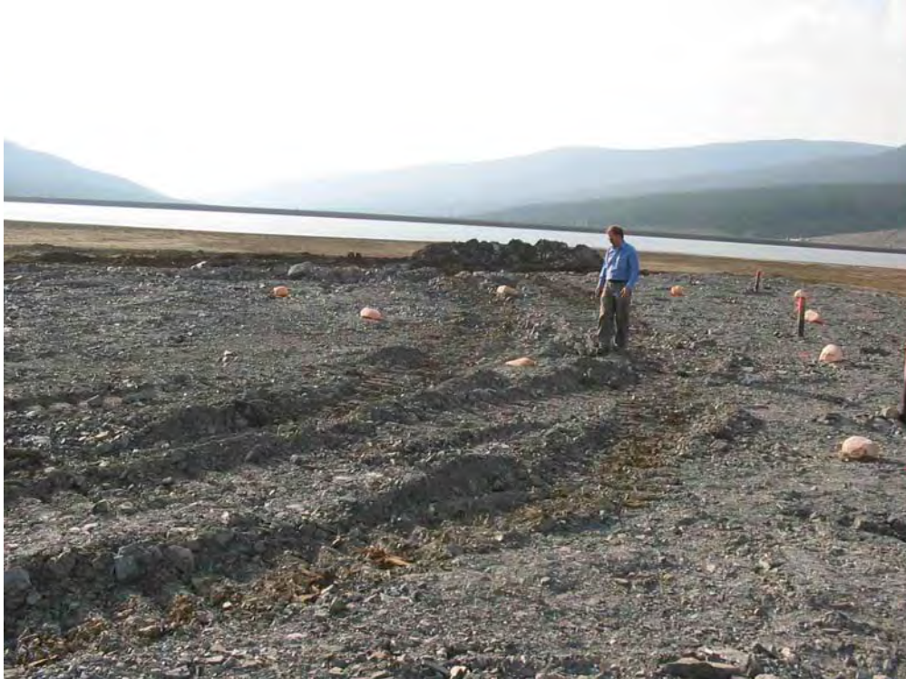
Figure 21. West test cover: Damage to surface of cover by equipment. Note disturbed marker stone in center.
