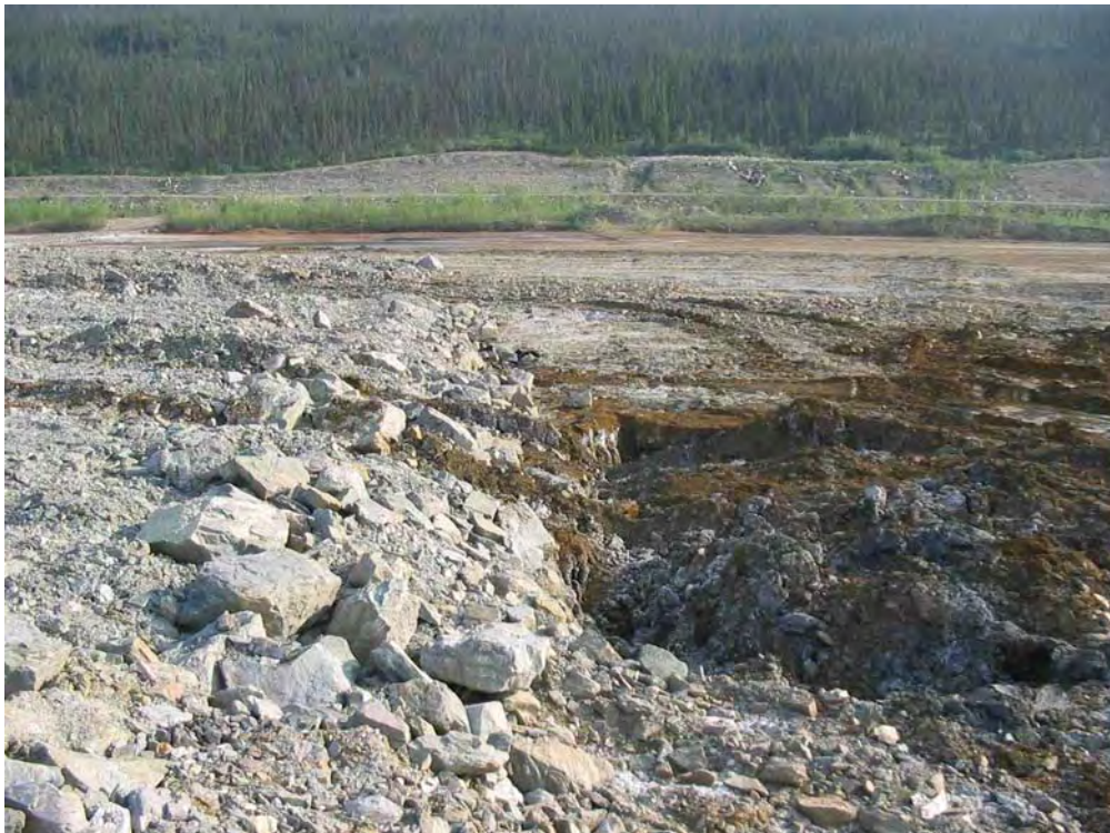
Figure 30. West test cover: Western edge, showing damage from equipment.
