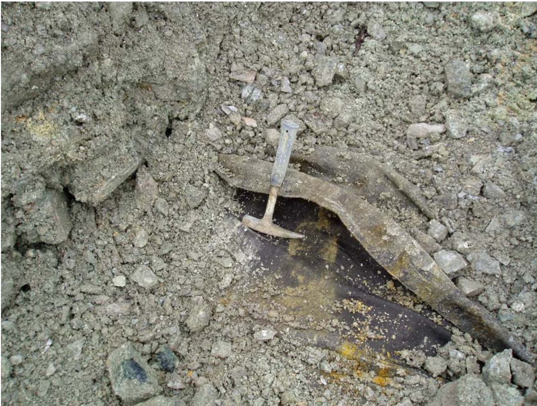
Photo 17: TP-TTC-04-06 Geotextile overlap showing no signs of tailings moving through the geotextile. The folds in the geotextile is as a result of rutting during construction caused by the trucks passing over the geotextile
