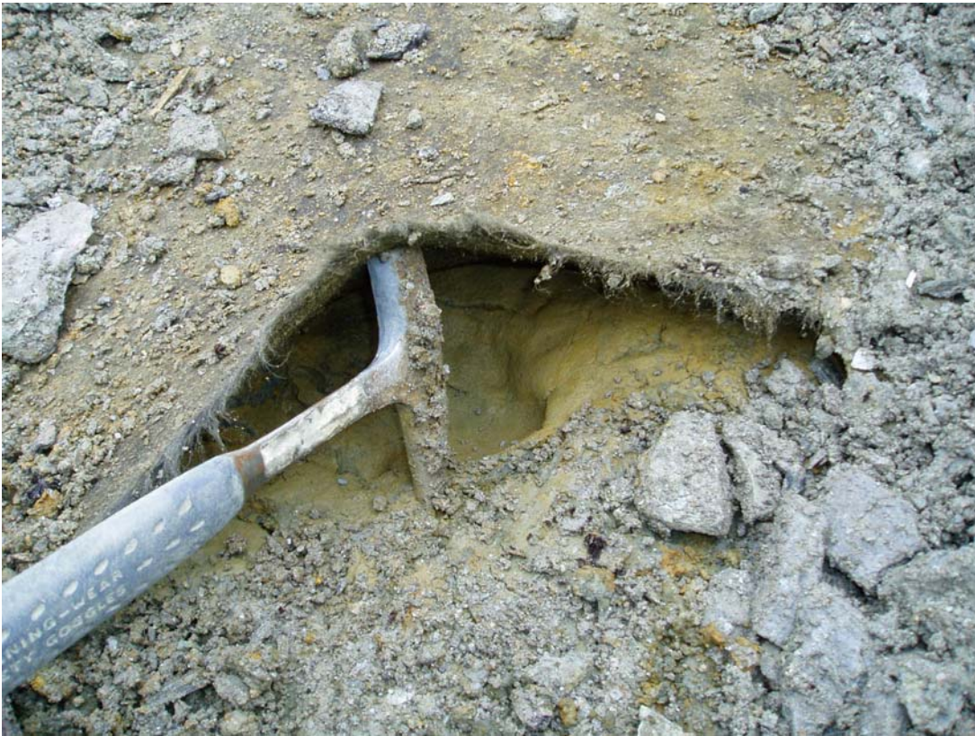
Photo 11: TP-TTC-04-04 Minor undulating surface at contact between cover material and tailings.
