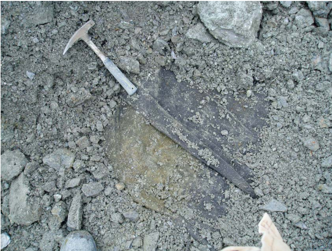
Photo 15: TP-TTC-04-05 Overlap section of the textile showing no signs of moving apart as a result of differential settlement. Also, no tailings are oozing through the seam opening.
