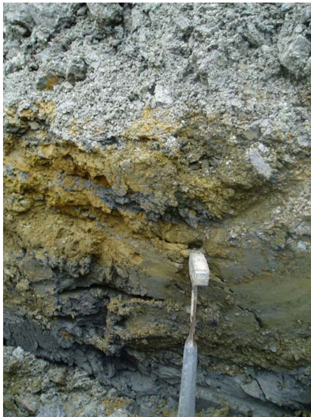
Photo 6: TP-TTC-05-02 View of the interface between the tailings and the waste rock cover.
