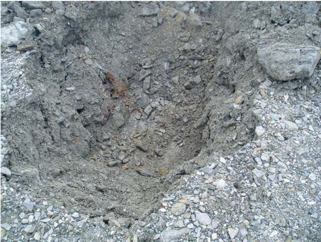
Photo 13: TP-TTC-05-05 Complete view of test pit showing the gradation of the cover material.
