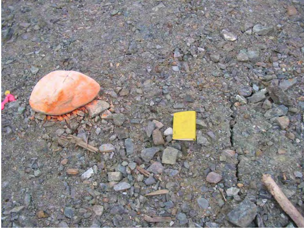
Figure 15. West test cover: Minor cracking near center of cover.
