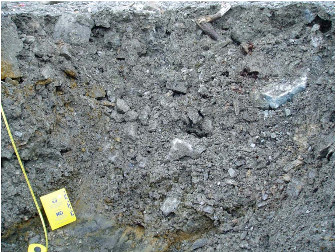
Photo 6: TP-TTC-04-02 Profile of test pit showing range of article sizes in cover material.
