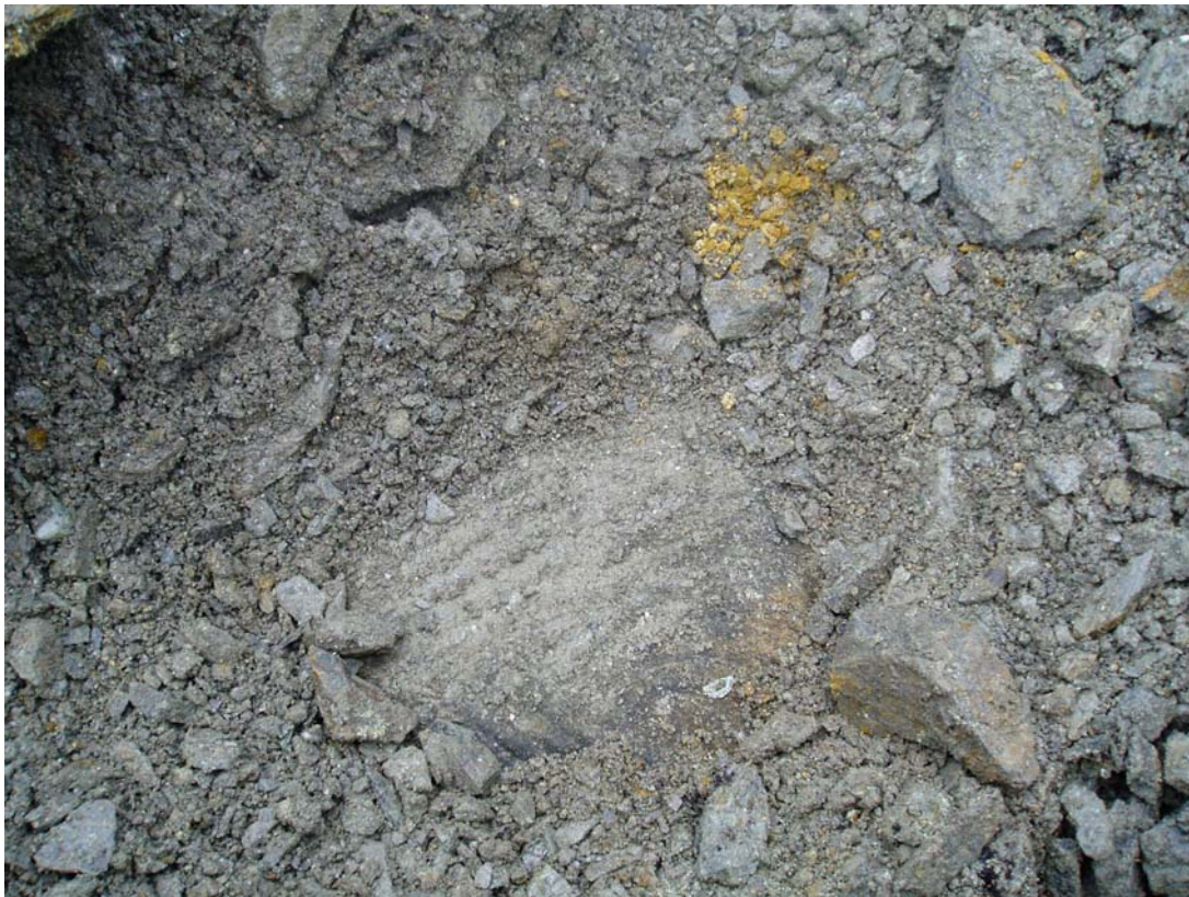
Photo 12: TP-TTC-05-05 The tailings has not migrated through the geotextile.
