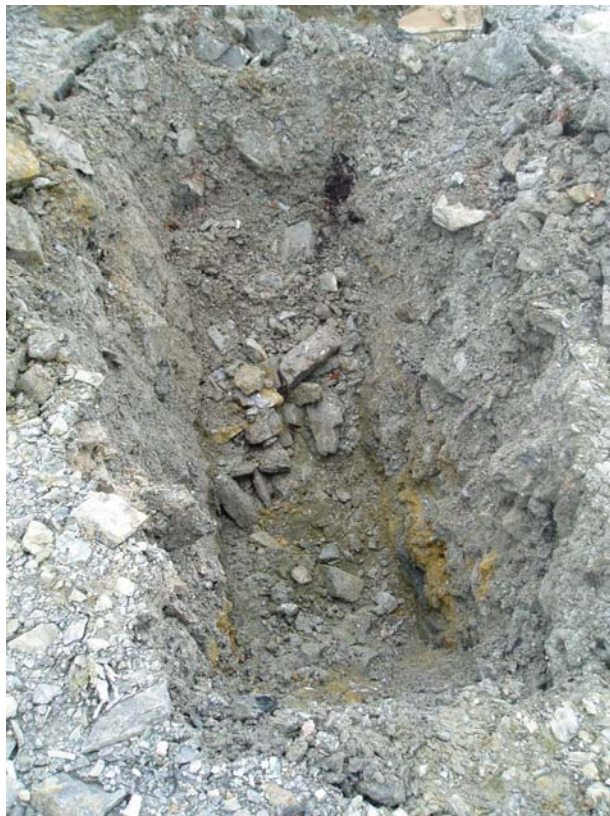
Photo 8: TP-TTC-05-03 View of complete test pit showing range in grain size from fines to boulders measuring 50 cm in diameter.
