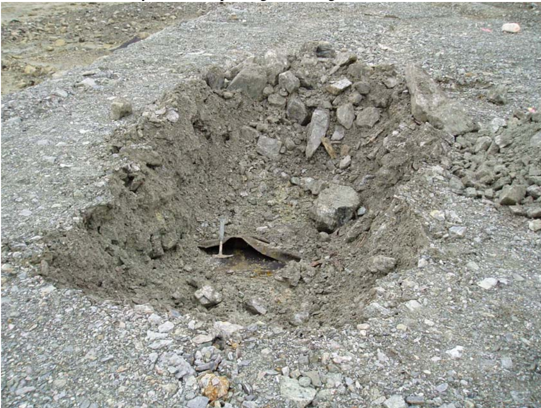
Photo 18: TP-TTC-04-06 Complete view of test pit showing range in gradation of cover material.
