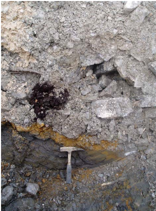
Photo 3: TP-TTC-05-01 Smaller scale view of the transition zone between tailings and the waste rock cover.
