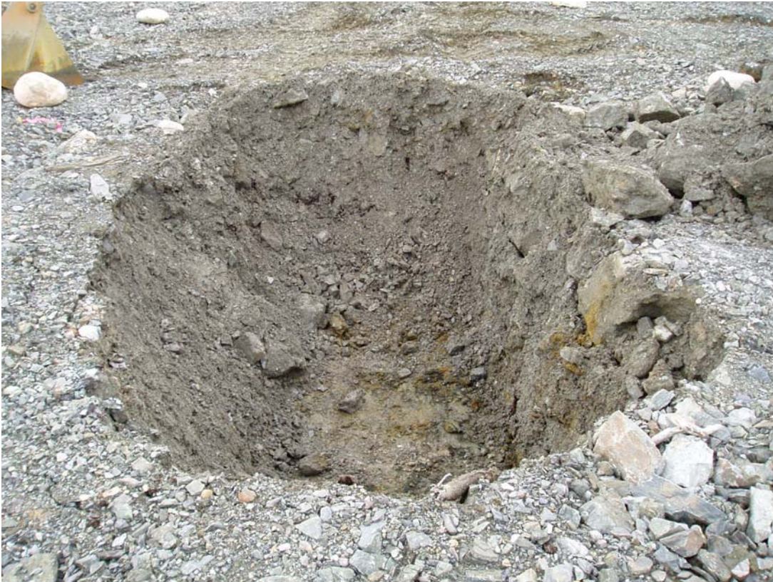
Photo 8: TP-TTC-04-02 Note the slope angle of the test pit walls. The material is very wet and the walls continuously caved in.
