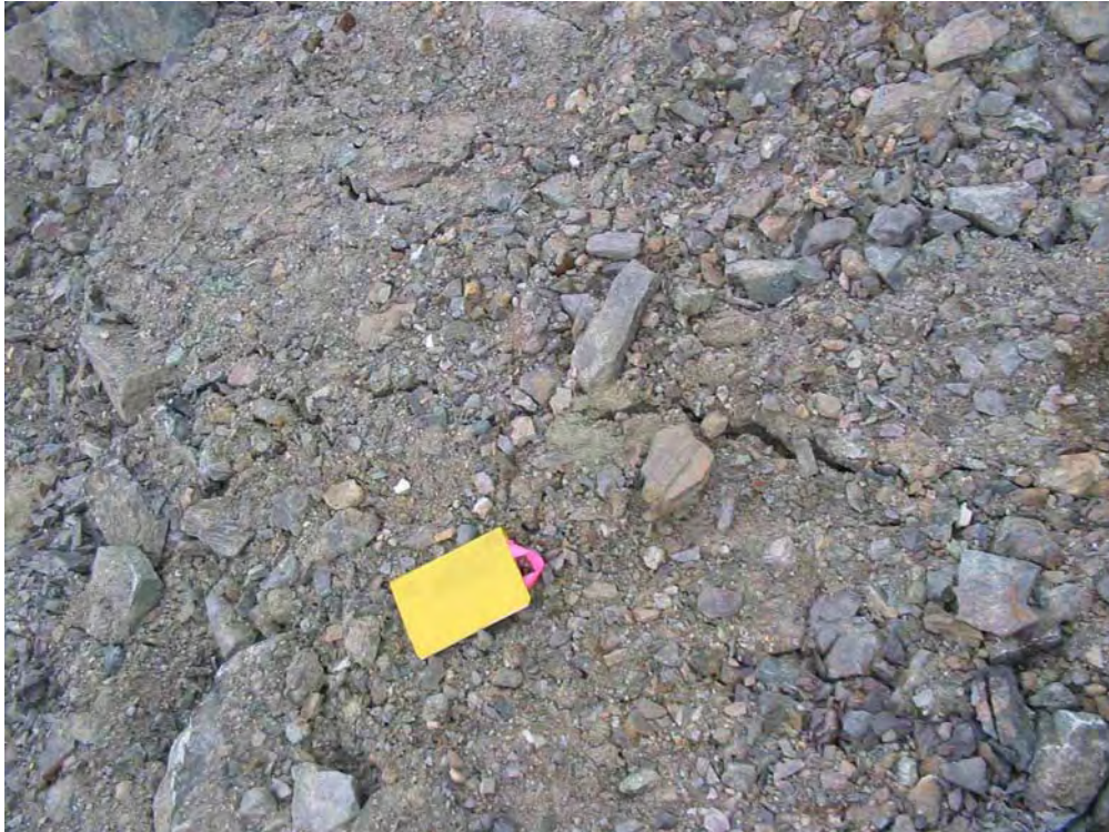
Figure 7. East test cover: Eastern edge, showing minor cracking.
