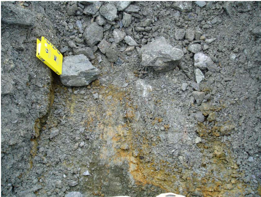
Photo 2: TP-TTC-04-01 Base of test pit excavation into tailings.
