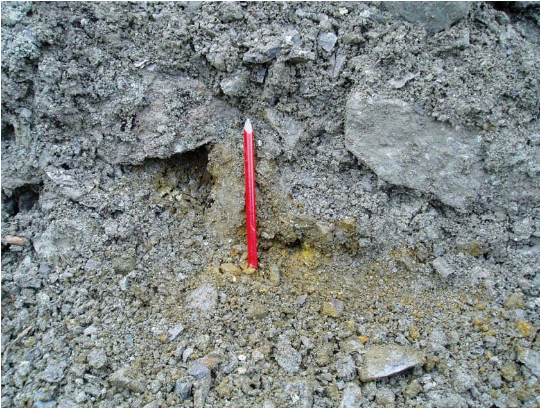
Photo 9: TP-TTC-04-03 Mixed zone of cover material and tailings of approximately 20 cm. The mixing appears to be dominated by larger boulders.
