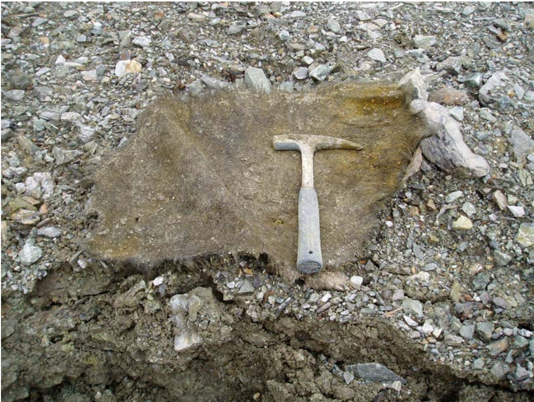
Photo 12: TP-TTC-04-04 The tailings has not migrated through the geotextile. Although both the tailings and the cover material were very wet, the geotextile was relatively dry.
