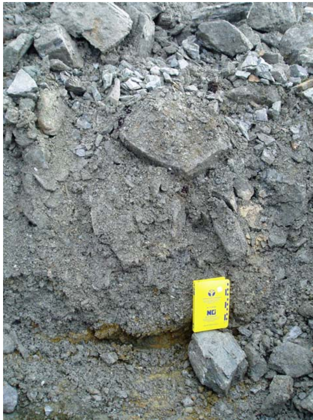
Photo 1: TP-TTC-04-01 Profile of test pit showing the undulated interface between tailings and cover material where mixing has occurred.
