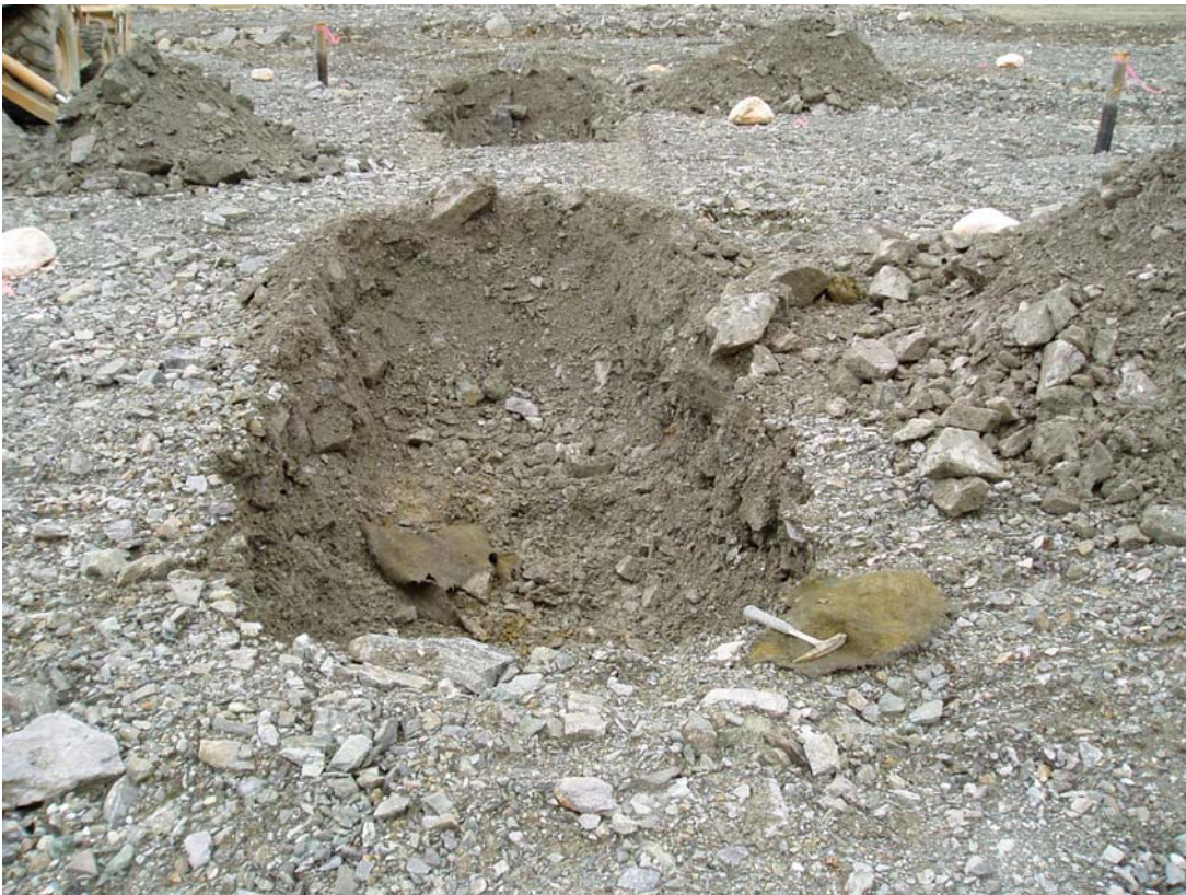
Photo 14: TP-TTC-04-04 Complete view of test pit showing the gradation of the cover material.
