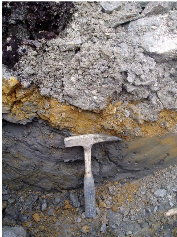
Photo 2: TP-TTC-05-01 Base of test pit excavation showing the interface between the tailings and waste rock cover. Note layer of oxidized tailings.
