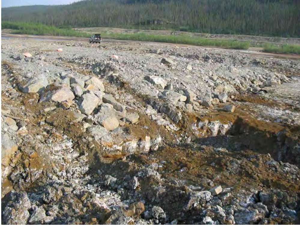
Figure 31. Western edge of west test cover showing equipment tracks in tailings and damage done to edge of cover by equipment.
