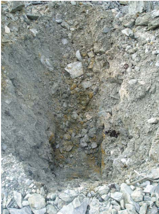
Photo 4: TP-TTC-05-01 View of complete test pit showing range in grain size from fines to boulders measuring 50 cm in diameter.
