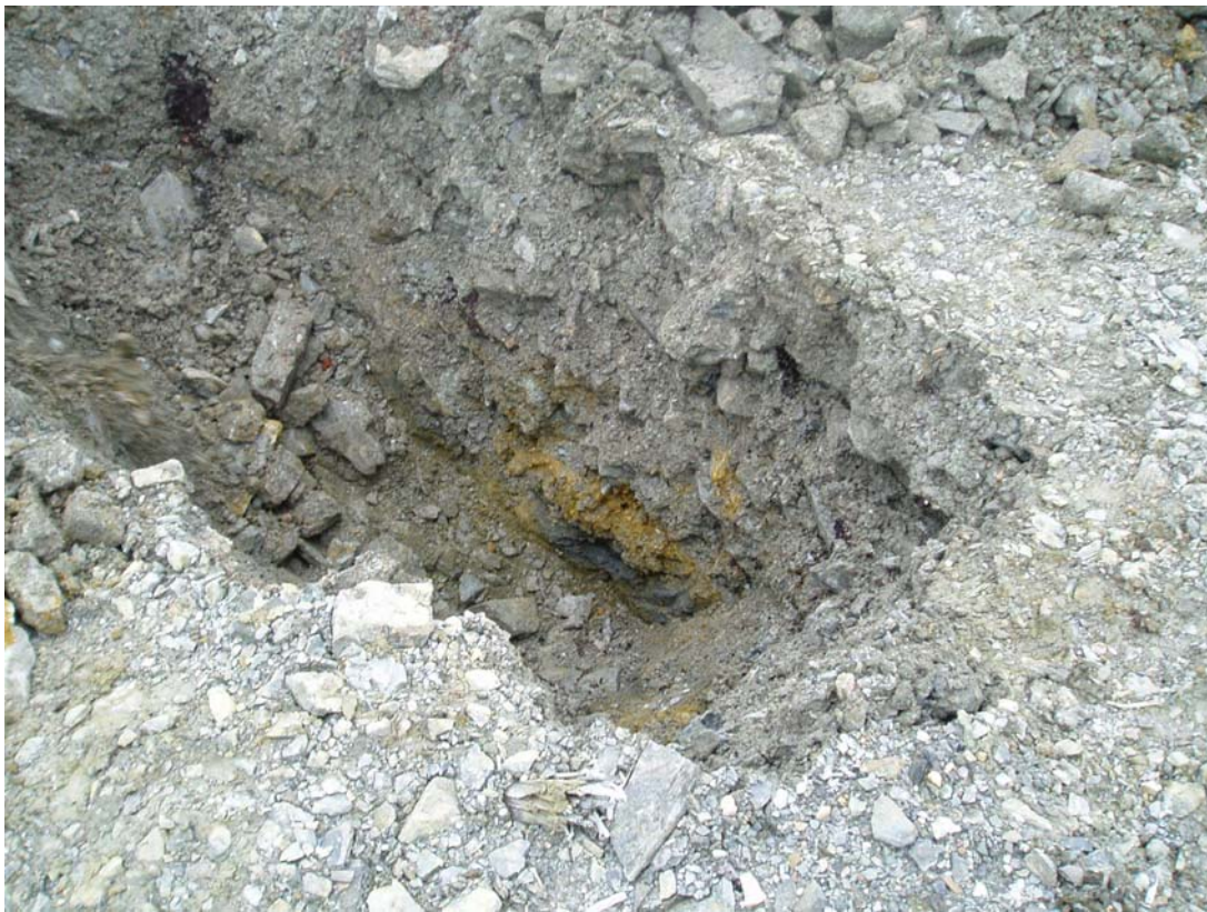
Photo 9: TP-TTC-05-03 Profile showing the range of particle sizes in the cover material.
