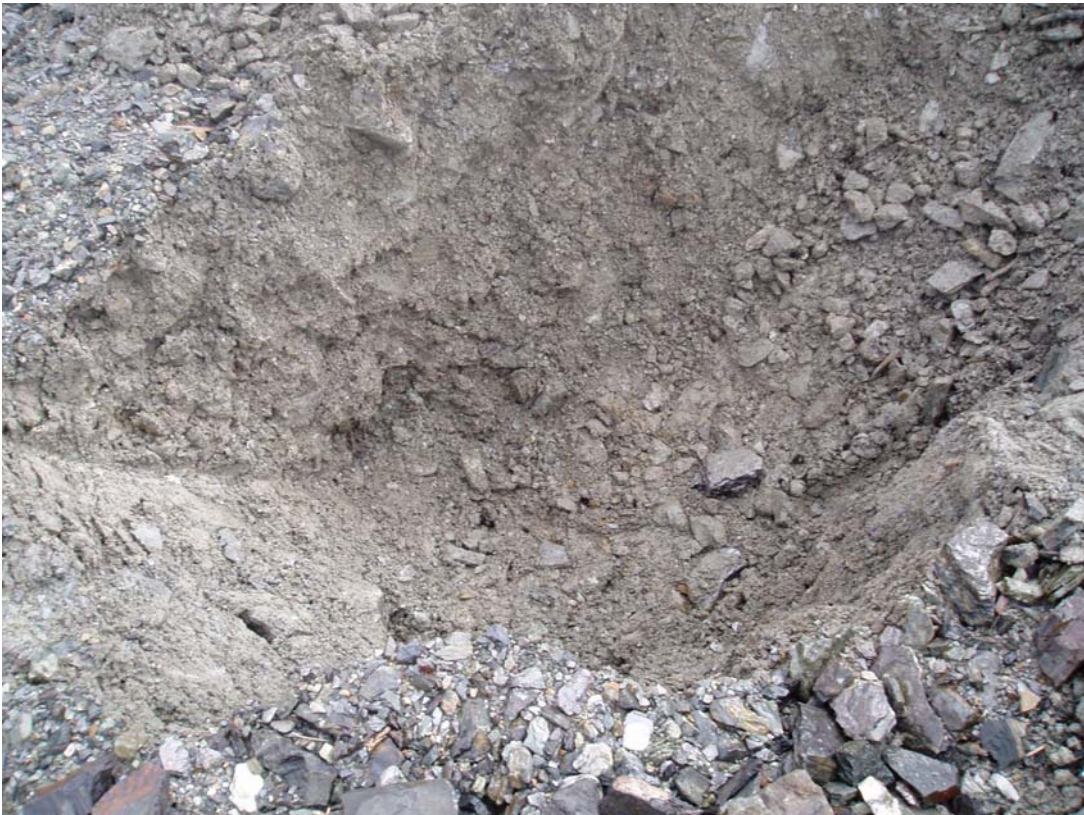
Photo 14: TP-TTC-05-06 The tailings has not migrated through the geotextile.
