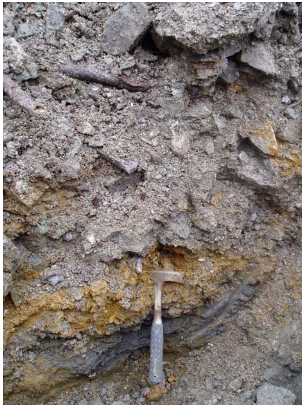
Photo 7: TP-TTC-05-03 profile of the test pit showing the interface between the tailings and the waste rock cover.
