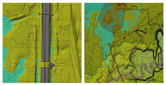
Figure 4.3. Example Computation Mesh with a Refined Channel and Break Lines for Embankments
