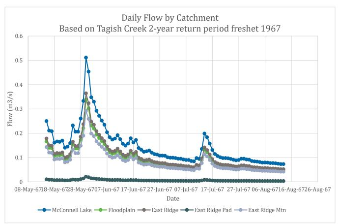
Figure 4.18. Hydrograph applied to Project area based on Tagish Creek 1967 2-year return period freshet.
