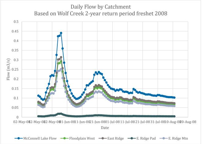
Figure 4.17. Hydrograph Applied to Project Area Based on Wolf Creek 2008 2-year Return Period Freshet.
