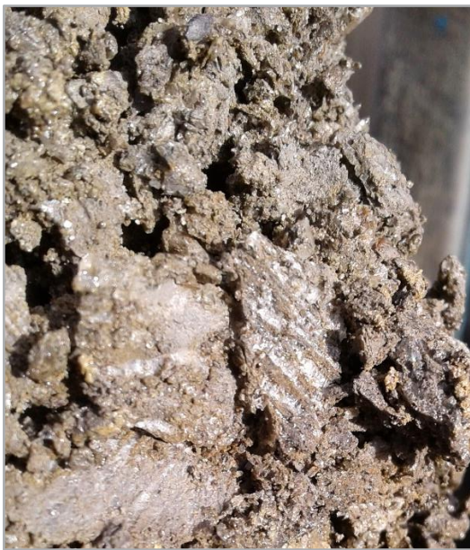
Figure 12: Visible Ice Lenses in Intact Section of Soil from Subsurface in Old Crow
