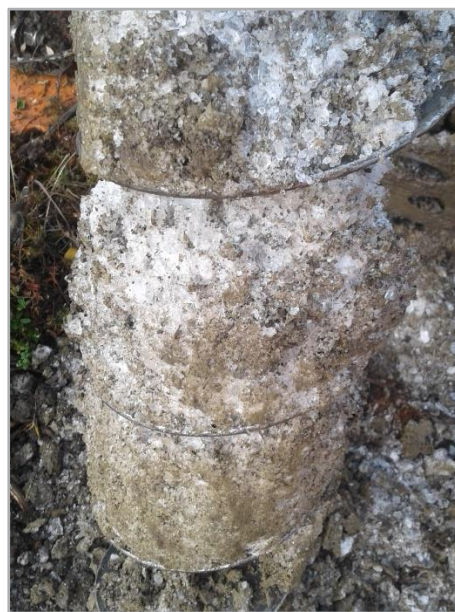
Figure 13: Ice Rich Interval Encountered during Drilling of Borehole in Old Crow.
