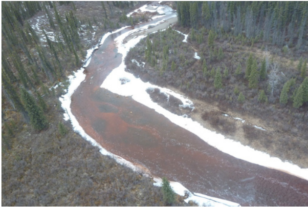
Rose Creek downstream showing metals deposition from acidic mine drainage from Faro Mine on Kaska traditional territory (Yukon Conservation Society, May 2017).
