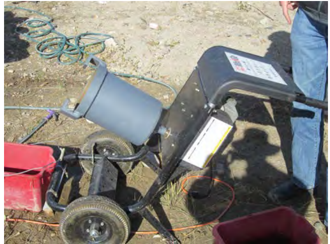
Figures 14 -17- Gavin Clarkson and the Portable Rod Mill Designed for Field Testing.
