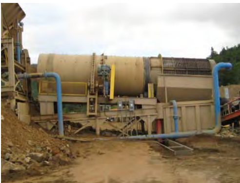
Figure 68 - High Speed Rubber Lined Trommel to Scrub Clay-Rich Gravels.
