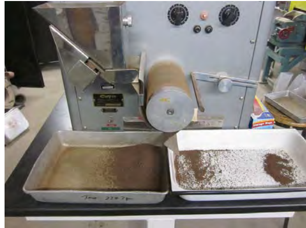
Figure 58 - Carpco Low Intensity Drum Magnetic Separator at UAF.
