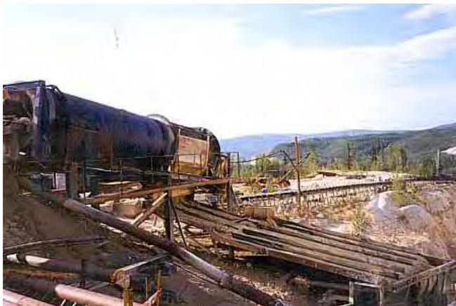
Figure 72 - High Clay Gold Recovery System Trommel Scrubber & Screen
