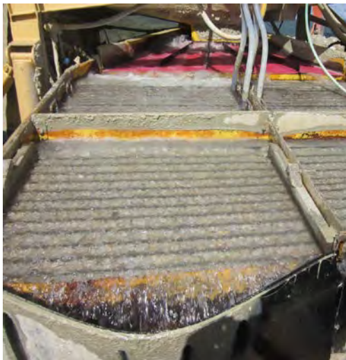
Figures 64 & 65 - Hard Packed Riffles in too Short of a Sluice Run.
