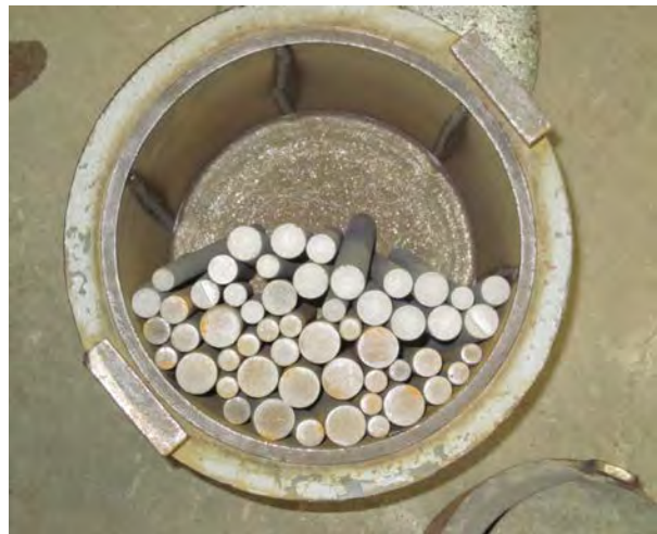
Figure 56 - 8" Diameter Rod Mill & Rods.
