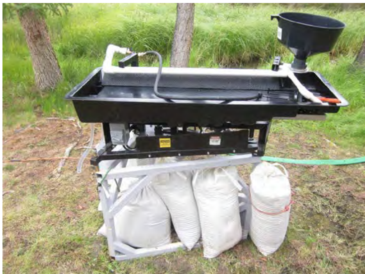
Figure 33 - Keene ST1 Shaking Table with Rotating Magnetic Separators with Simple Feeder Mounted on Steel Base with Sand Bags.
