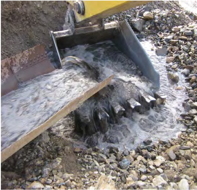
Figure 48 - Test Sluice Concentrates were hand panned to raw gold where possible or to a final concentrate for later lab testing. Gold samples were cleaned dried and weighed.
