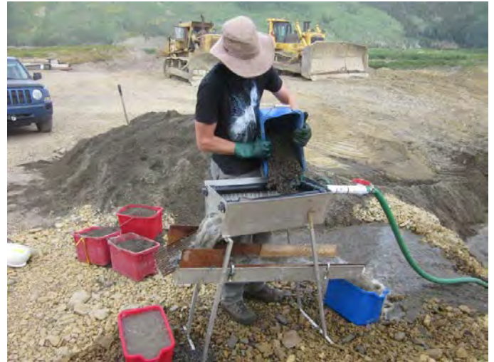
Figure 47 - Gavin Clarkson Processing Sluicelox Tailings Sample on Author's Testing Sluice.
