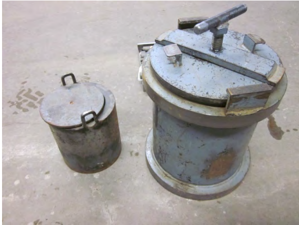
Figure 57 - Rod & Ball Mills Used in Tests at UAF.
