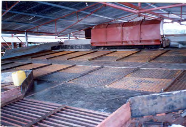
Figure 70 - Above - Good Design with Hydraulic Riffles at Top and Slick Plates between Sections of Coarse Expanded Metal Riffles.
