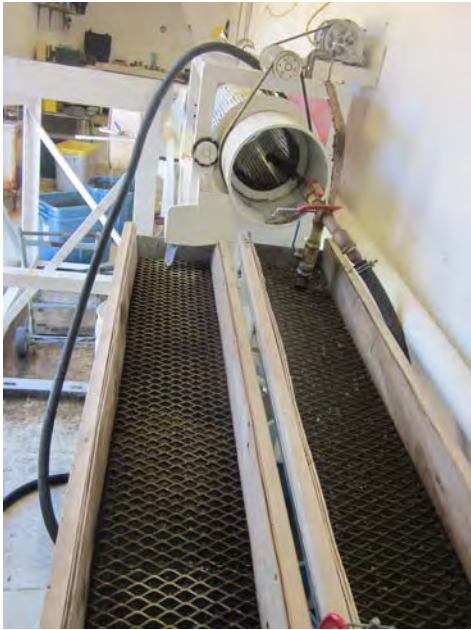
Figure 22- Conventional Long Tom with Trommel.
