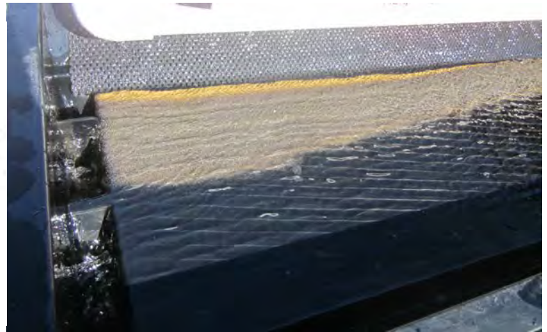
Figures 30 & 31 - Schematic (Burt, 1987) and Photo of Deister Type Shaking Table Deck: Particle paths of high density (dark) and low density (light) particles on a concentration table. Note the band of very fine gold on the top of the Keene table and the band of high density minerals in the middle of the table (middlings). In this photo there are no low density minerals to be directed to the slimes or tailings as shown in the schematic.
