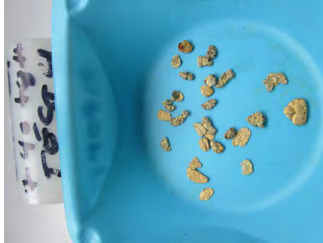
Figure 82 - +8# Gold Nuggets & Flakes Recovered by Grinding a Concentrate with Abundant Garnet.
