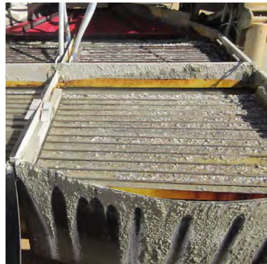
Figures 64 & 65 - Hard Packed Riffles in too Short of a Sluice Run.
