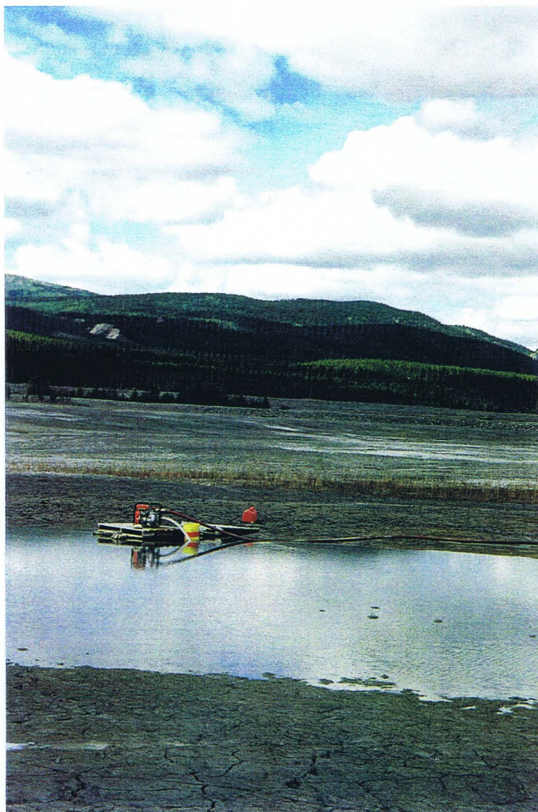
Photograph 5. High pressure pump delivers 300 liters water per minute for irrigation.
