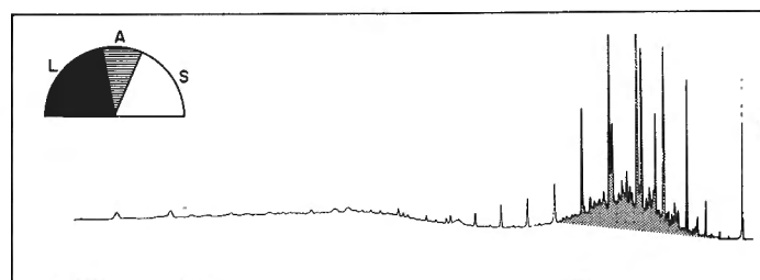
FIGURE 4-8. Examples of Type 2 contamination of rock extracts.
