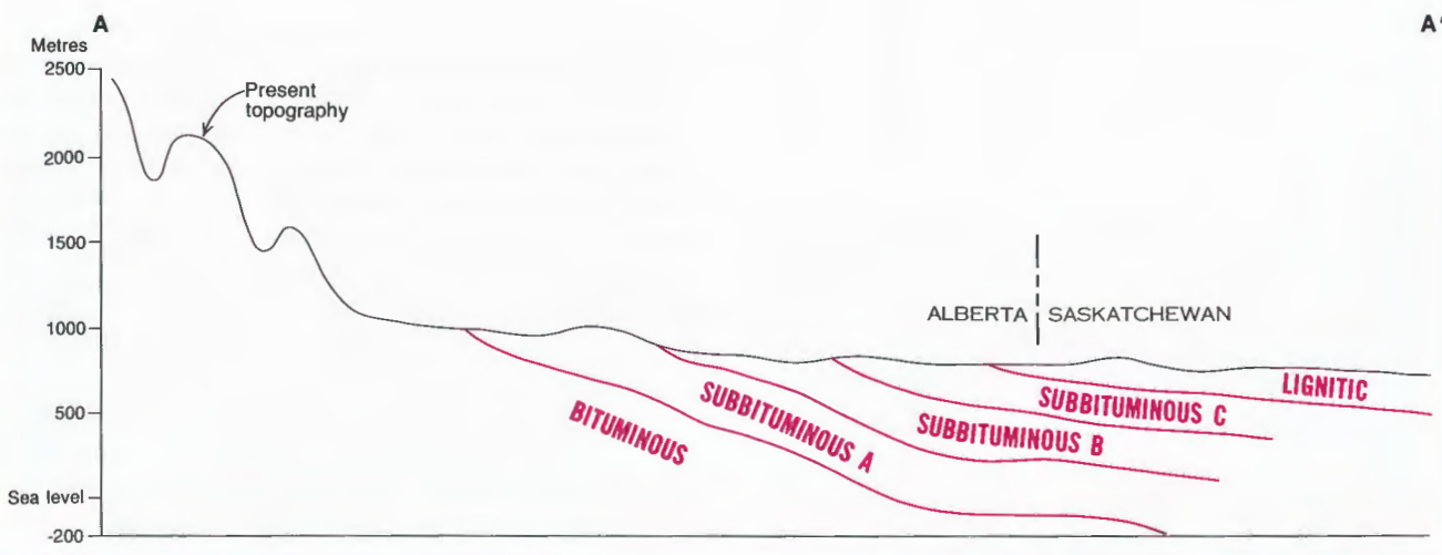
Figure 7.4. Regional rank distribution of near-surface coals in the Interior Plains (from Steiner et al., 1972; Nurkowski, 1985).
