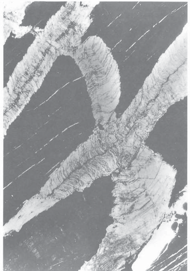
Figure 68. Quartz veins with fibrous fill. Two sets of quartz veins with fibrous vein-fill. Note the curved nature of the fibres.
