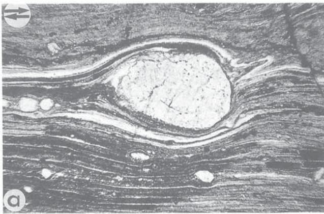
Figure 65. Quarter structures. Different types of structures develop in the quarters (Fig. 64) in the matrix adjacent to stiff inclusions, according to the angular relations between the local perturbed flow and the foliation/layering in the matrix. In a bulk coaxial flow, the foliation/layering of the matrix in all four quarters would be subjected to layer normal shortening. However, in bulk noncoaxial flow, the perturbed local flow is asymmetrically disposed about the stiff inclusion in a manner which directly reflects the sign of the vorticity of the bulk flow in the matrix (see Fig. 64). The examples shown here are observed in the XZ plane of the finite strain ellipsoid. The sense of shear along the shear plane, and in C the extensional and shortening quadrants of the flow, are shown.
