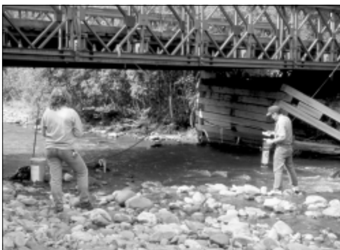
Figure 5. "Waterpod" instruments were mounted on existing structures, such as bridges, whenever possible.
