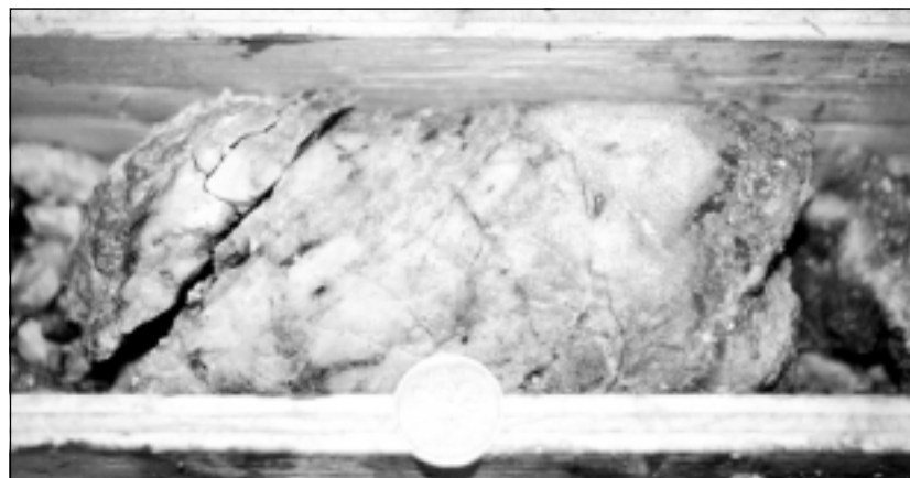
Figure 18. Quartz-sulphide mineralization typical of veins from the Flex zone at the Mount Nansen mine.
