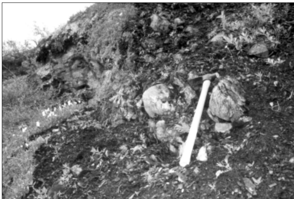
Figure 33. Limestone balls mark the immediate footwall to the Ni-Zn-PGE horizon in the MM grid extension area on the Taiga property.
