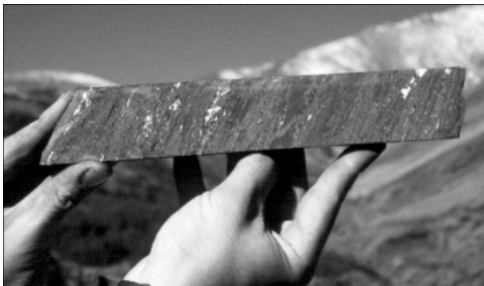
Figure 25. High-grade massive sulphide core from the Wolf property.
