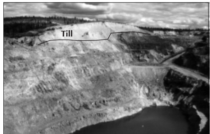
Figure 9. Vangorda mine looking to the southeast. A blanket of till is visible on the pit wall in the background. The till depth varies from 1 m to 50 m.
