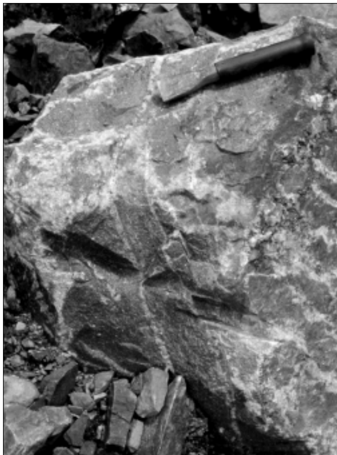
Figure 7. Sheeted arsenopyrite-rich quartz veins (white) cutting a lamprophyre dyke (dark) in the Saddle area. Chisel near top is 21 cm long.
