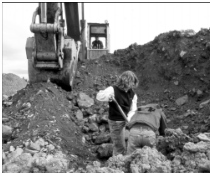
Figure 2. Pay gravels and feed materials were sampled for grain-size analysis and gold content.
