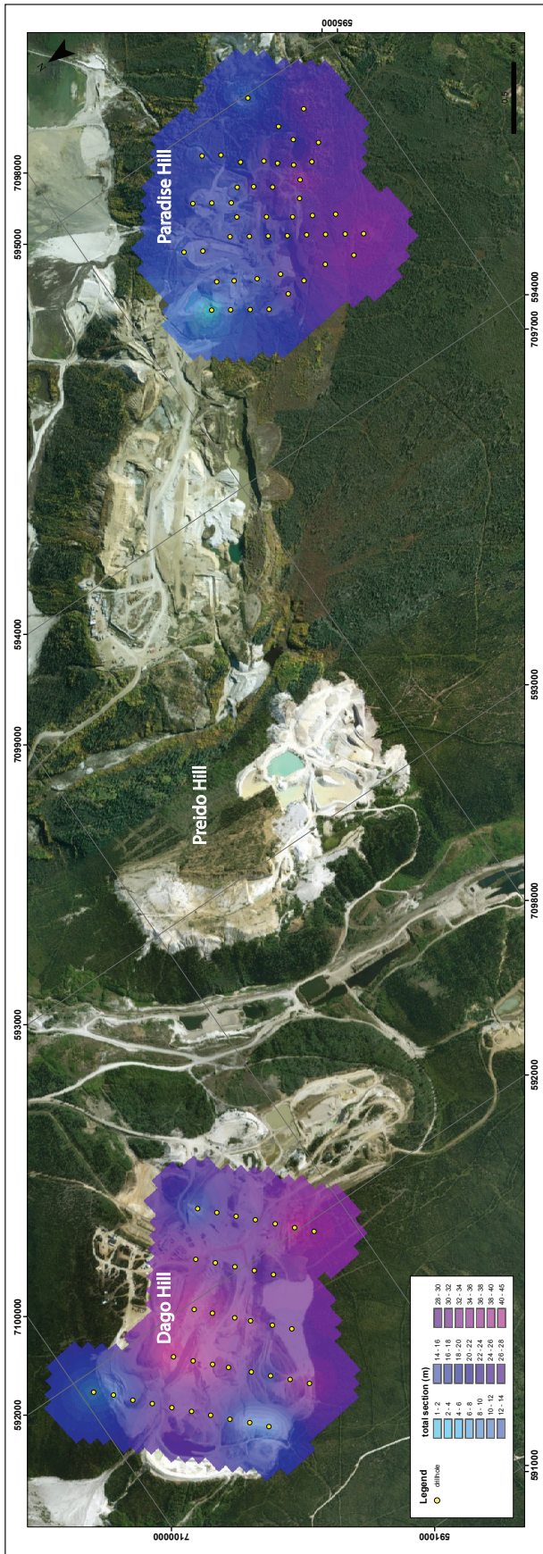
Figure 6. Satellite image of Dago Hill and Paradise Hill on lower left limit Hunker Creek, overlain by a raster image of total section thickness (gravel and overburden).
