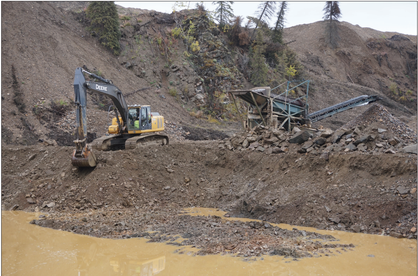
Figure 5. M2 Gold Mines operation on the Sixtymile River. After a thin layer of uneconomic gravel is stripped off, a single excavator can handle the bulk of the mining operation. In this cut, the excavator digs pay and feeds the plant. As the excavator moves along the mining face it drags the trommel in order to maintain the appropriate feed spacing.
