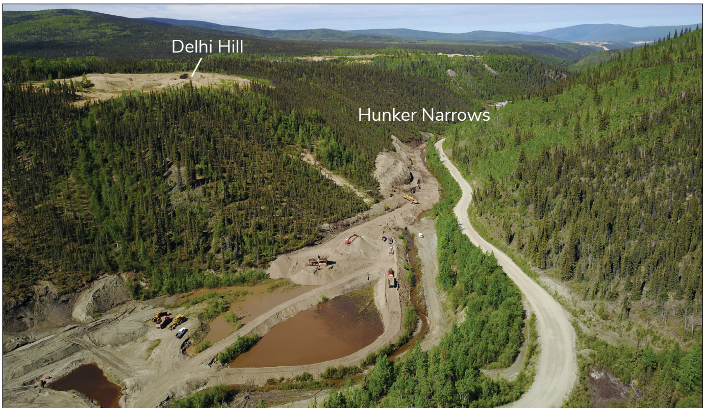
Figure 4. A view looking downstream on Hunker Creek toward the Hunker Narrows. The former White Channel gravel pay streak was only partially left on Delhi Hill. The remainder was eroded onto the rim of the hill and into the valley bottom.
