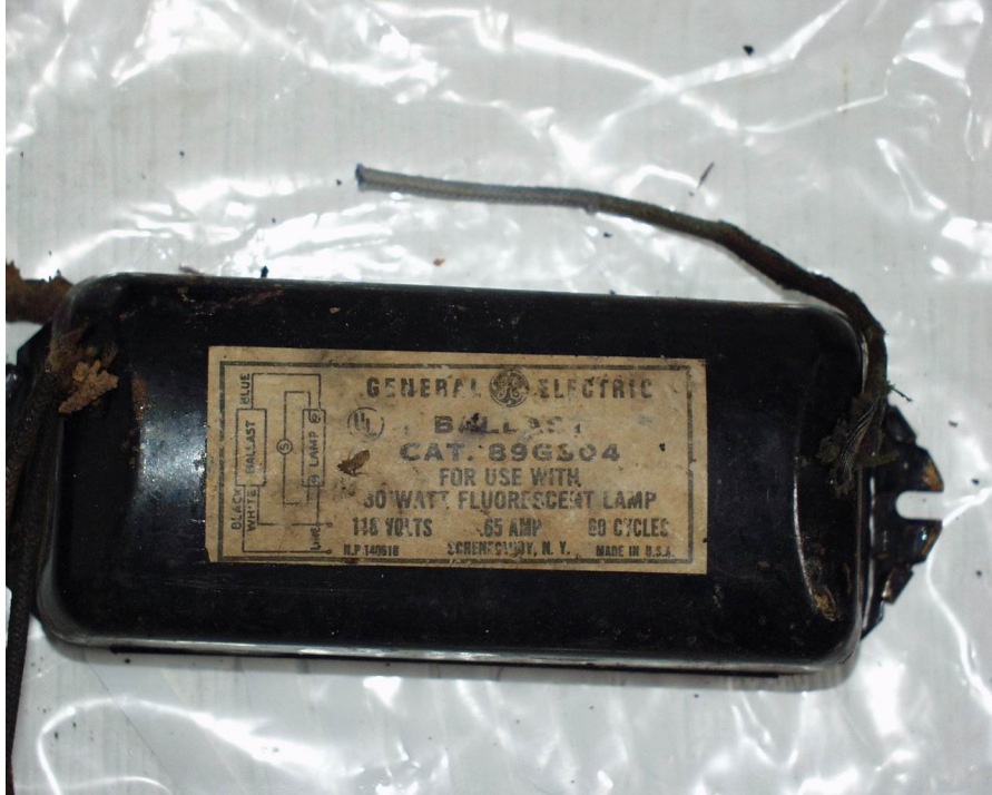
Fig. 4 Fluorescent light ballast
