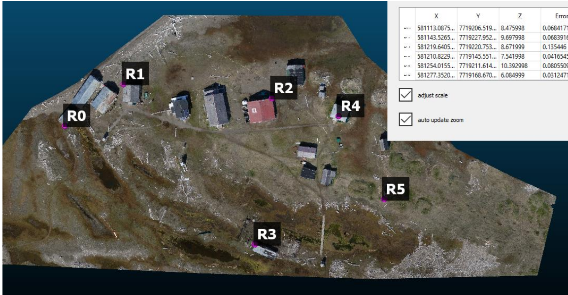
Figure 35 Alignment points for the Study Area 1 re-alignment. The cloud shown here is the reference cloud. © Katelyn O'Keefe, 2022.
