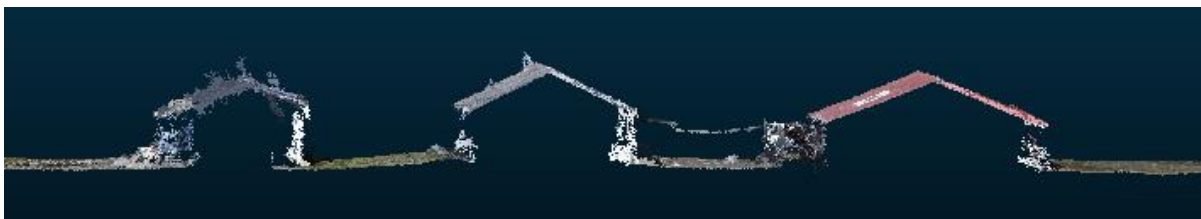
Figure 36. Cross-section of the aligned Study 1 point clouds. No gaps between the point clouds can be seen, suggesting proper alignment. © Katelyn O'Keefe, 2022.
