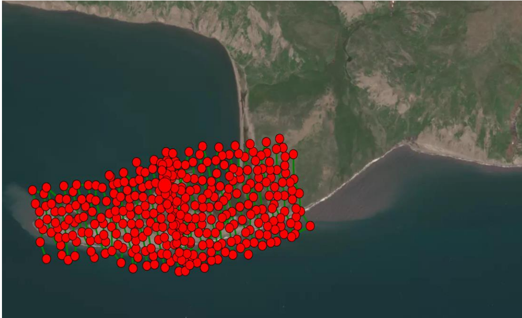
Figure 28. Flight plan for dataset Pauline Cove 2019. Each red dot is the location of a geolocated image. Image generated using Pix4Dmapper©..© Katelyn O'Keefe, 2022.
