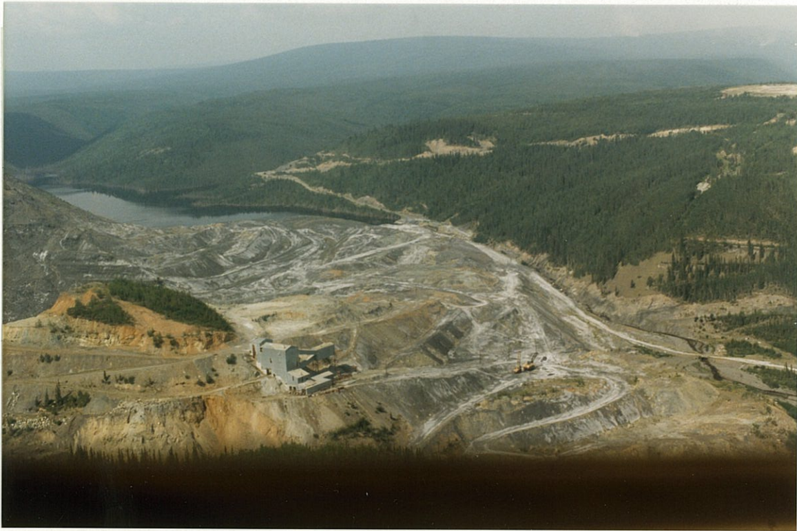
Photo 3: Clinton Creek waste dump, looking upstream toward Hudgeon Lake. Open pit is at left, crusher in foreground, and concentrator site on plateau at upper right. July 1986.
