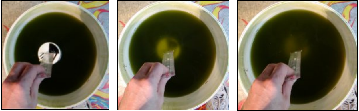
Figure 2. Secchi depth measurement for algal cultures.
