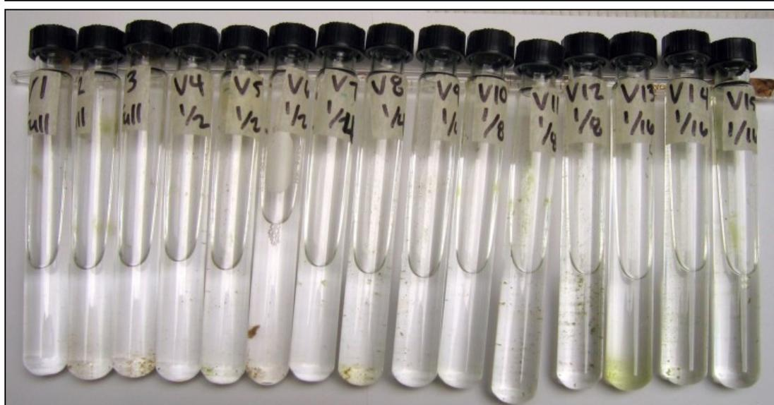
Figure 5. Algal growth at the end of toxicity threshold test. Note mix of attached and planktonic growth.
