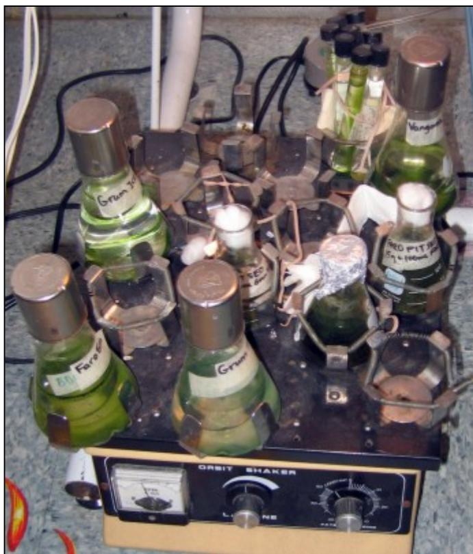
**Figure 1. Algal cultures in shake flasks on orbital shaker.**
