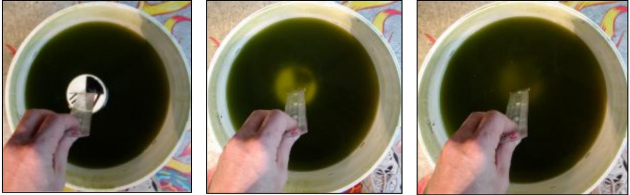
**Figure 2. Secchi depth measurement for algal cultures.**
