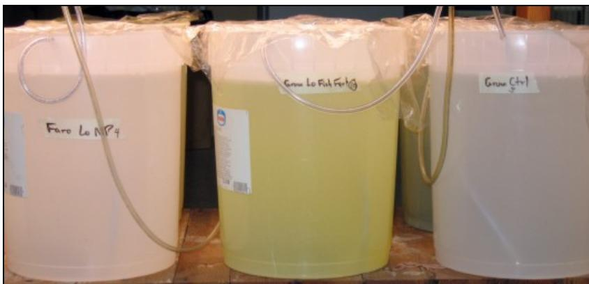
**Figure 17. Algal growth in Grum low fish fertilizer treatment. Notice the absence of growth on the walls of the container. Taken on Week 6.**
