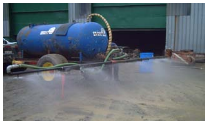
Spray Pattern of Nozzles
