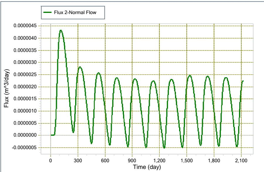
Daily flux rates through the bottom of capillary break layer.
