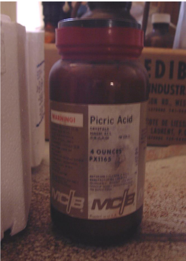
Fig. 1 – Container of picric acid (trinitrophenol) in assay lab chemical storage in First Aid building.
