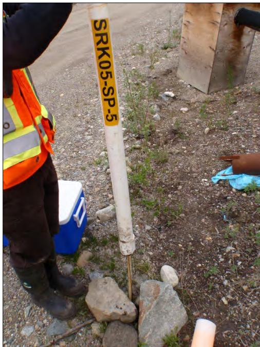
**Photo 14:** View of well SRK05-SP-5. Well broken at surface upon arrival. Large amounts of soil found on waterra tubing already existing in well. Photo taken on June 20, 2014.
