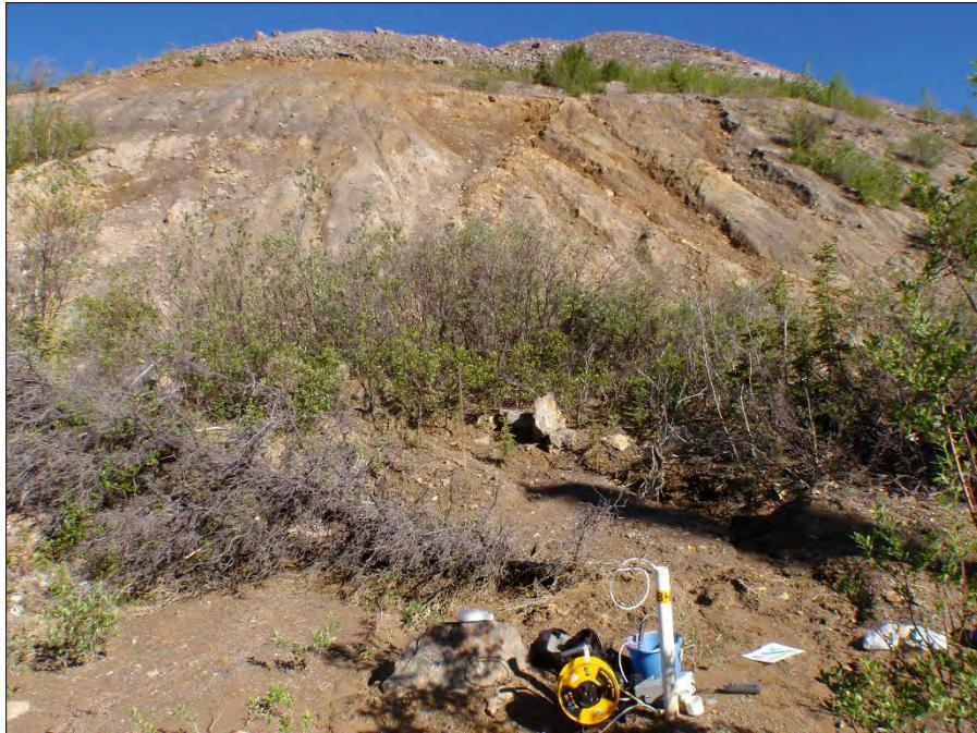
**Photo 2:** View of wells BH14A and BH14B. Background shows a slide which has partially buried BH14A, leaving a stick-up of 0.02m. Photo taken on June 19, 2014.
