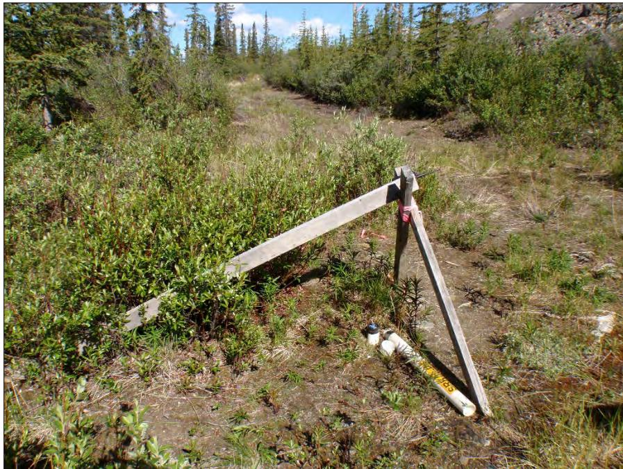
**Photo 5:** View of well SRK08-P9. Stick-up broken upon arrival. Photo taken on June 19, 2014.
