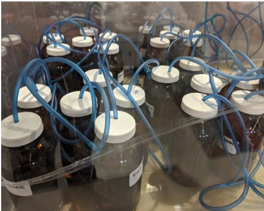
Figure 4-3: Anoxic Aging Test Setup
