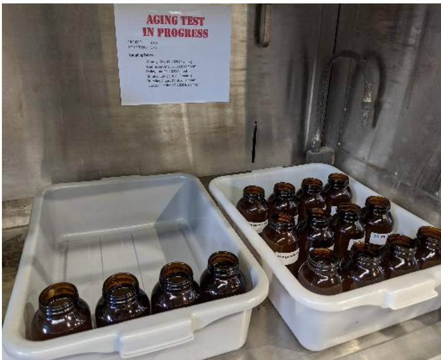
Figure 4-2: Oxic Aging Test Setup
