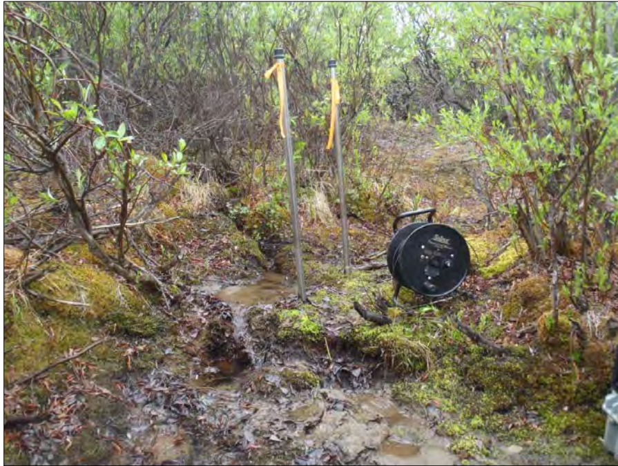
Photo 1: View of drive point wells GSI-DC-01A and GSI-DC-01B. Photo taken on June 1, 2015.
