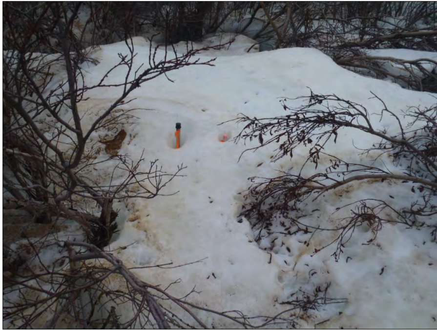
Photo 3: View of drive point wells GSI-DC-03A and GSI-DC-03B. Photo taken on June 2, 2015. Drive point wells are frozen beneath accumulated ice.
