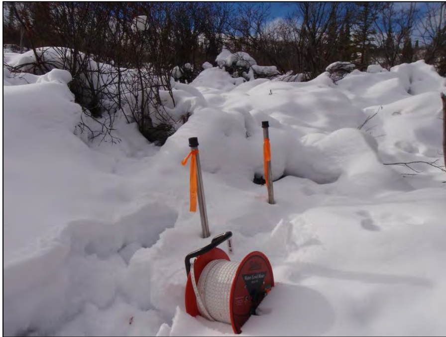
Photo 1: View of drive point wells GSI-DC-01A and GSI-DC-01B. Photo taken on March 18, 2015.
