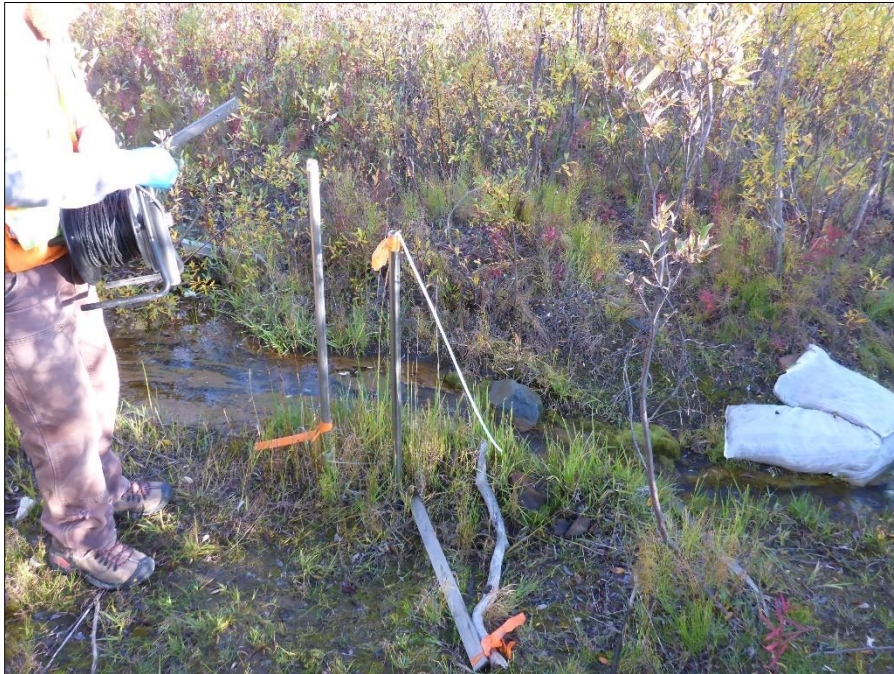
Photo 2: View of drive point wells GSI-DC-02A and GSI-DC-02B. Photo taken on August 29, 2016.
