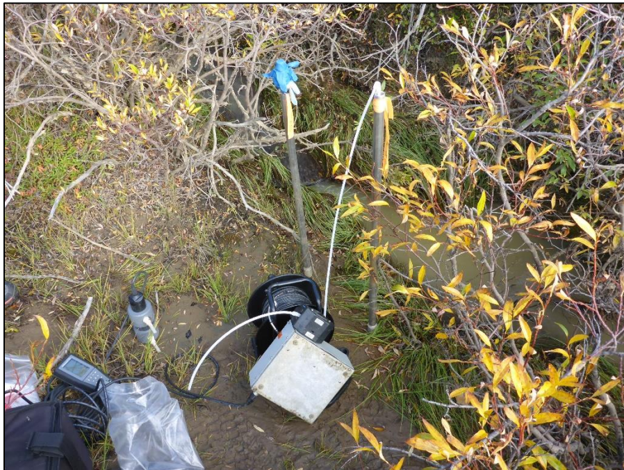
Photo 26: View of drive point wells GSI-PC-03A and GSI-PC-03B. Photo taken on August 31, 2016.
