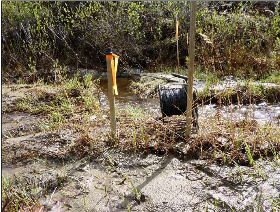
Photo 5: View of drive point wells GSI-DC-06A and GSI-DC-06B. Photo taken on May 26, 2016.
