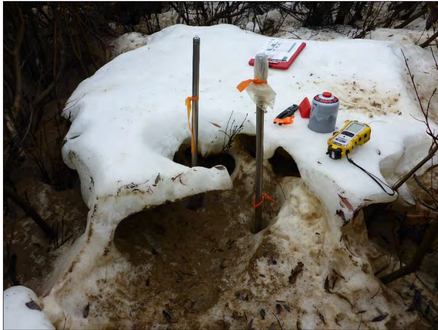
Photo 3: View of drive point wells GSI-DC-03A and GSI-DC-03B. Photo taken on May 25, 2016.
