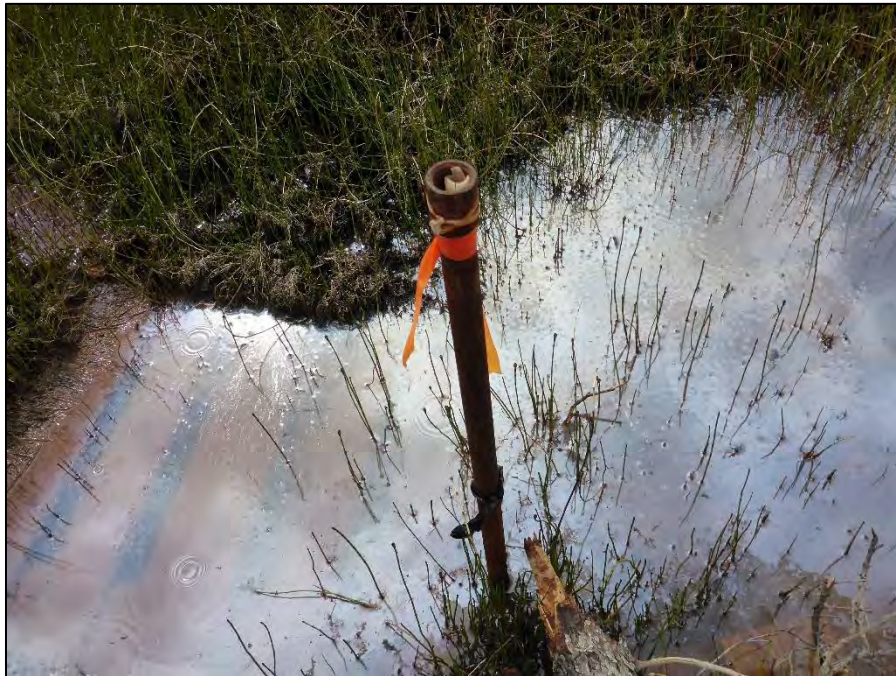
Photo 38: View of drive point well MP09-14. Photo taken on May 26, 2016.
