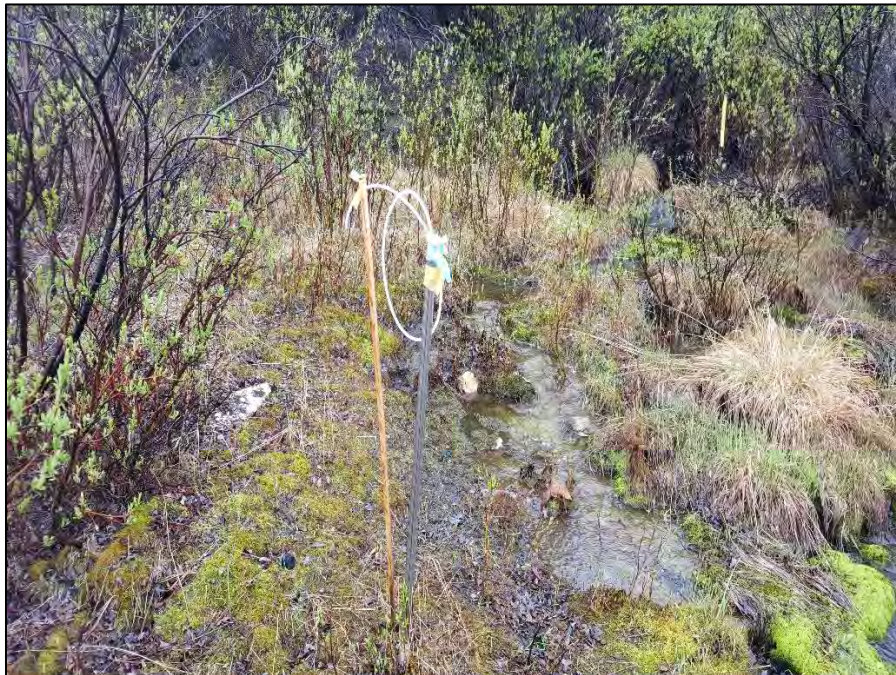
Photo 12: View of drive point well GSI-HA-03A. Photo taken on May 25, 2016.
